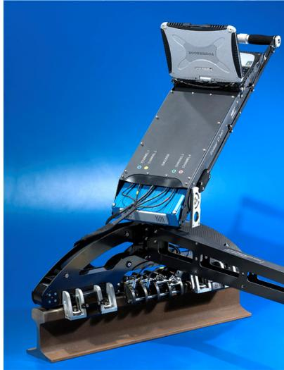
*Figure 2: Push Trolley for Manual Railway Inspection*
