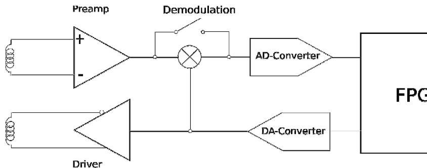
Figure 1: Block Diagram of one Eddy-Current Channel
