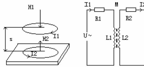
FIGURE 1. TESTING PRINCIPLE AND THE EQUIVALENT CIRCUIT
