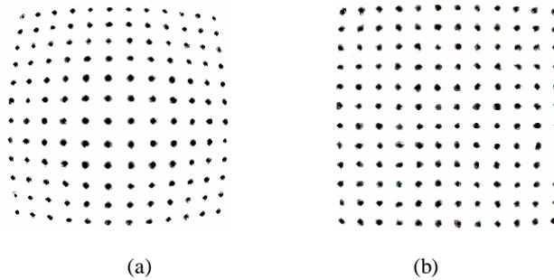
Figure 6. Image of the calibration template, (a) Distorted image. (b) Corrected image.
