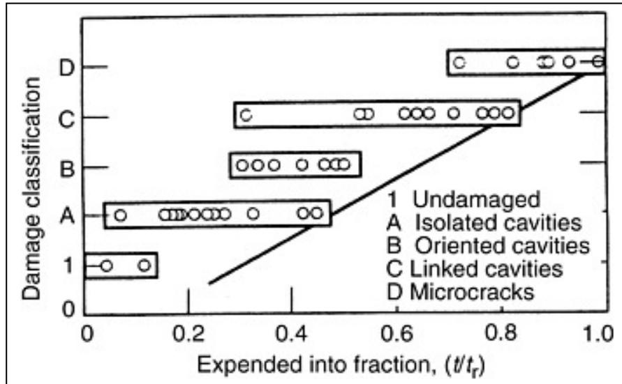
Figure 6 Creep failure curve and Neubauer<sup>[1]</sup> damage classification.
