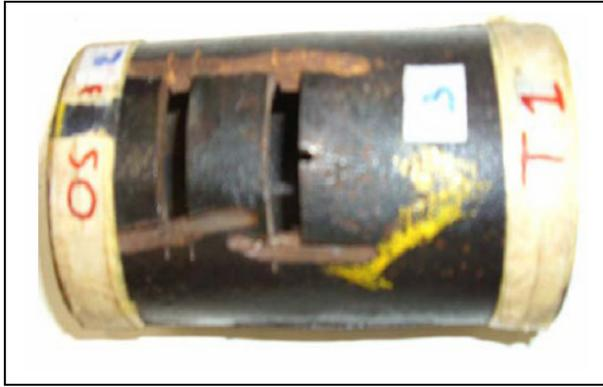
Figure 2: Regions after visual exams shows the start and end point of failure.
