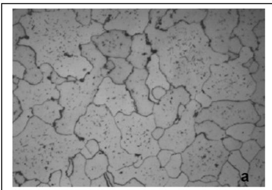
Figure 4: Sample T1 showing creep damage level "A" and "B" according Neubauer<sup>[1]</sup>.
