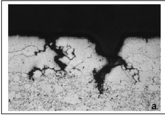
Figure 5: Sample T2 showing creep damage level "C" and "D" according Neubauer<sup>[1]</sup>.
