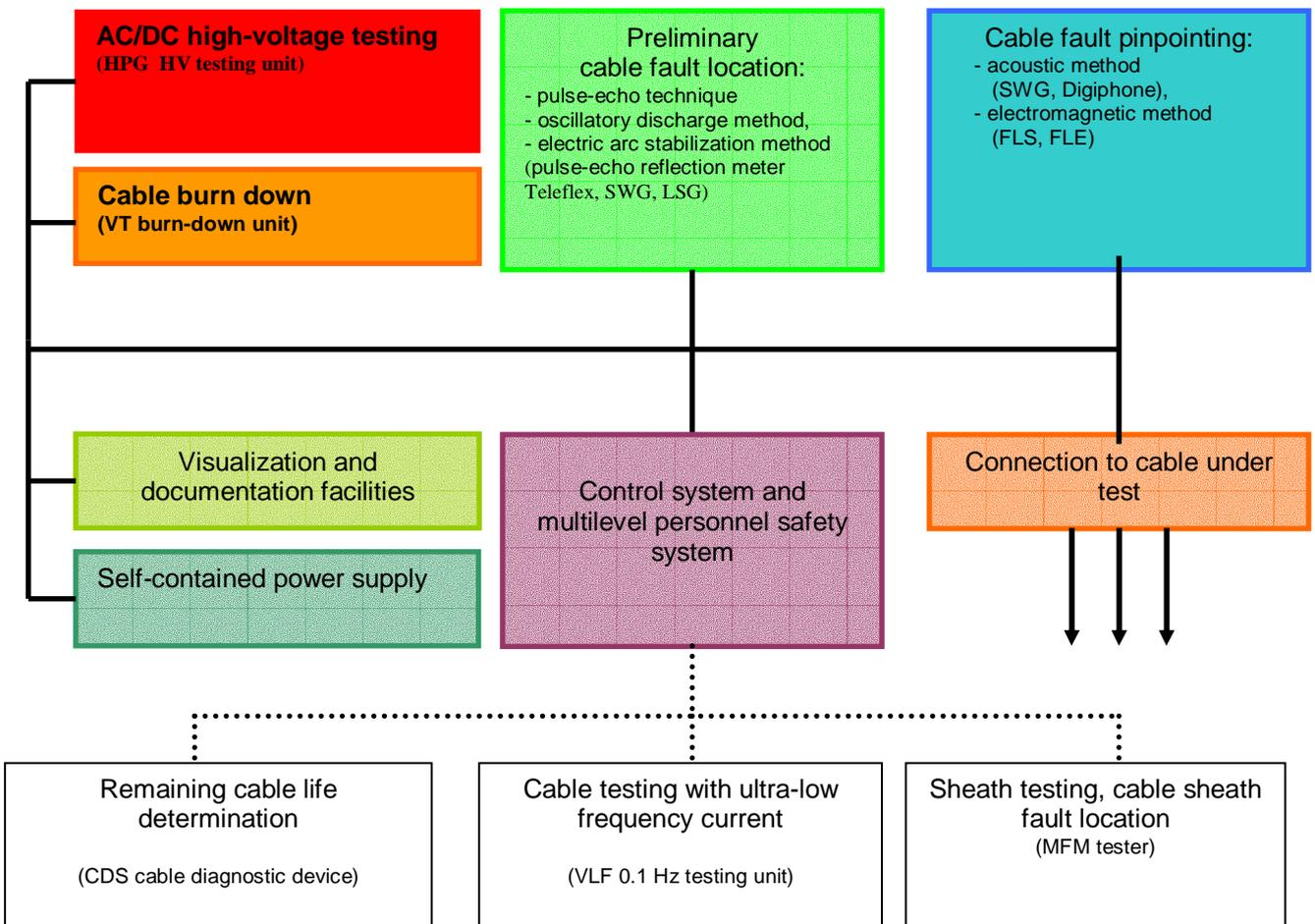
**Fig.11. Functional Chart of the Laboratory for Power Cable Fault Location and High-Voltage Testing**
