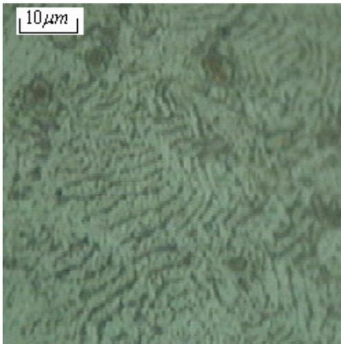
(a) magnetic domains of 20steel specimen without load after annealed
