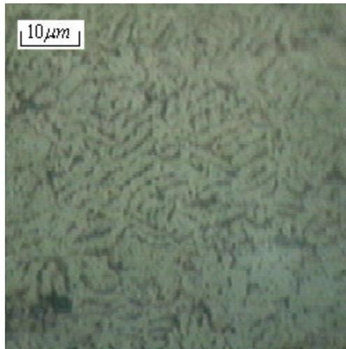
(b) magnetic domains of 20steel specimen exerted by 50kN load after annealed
