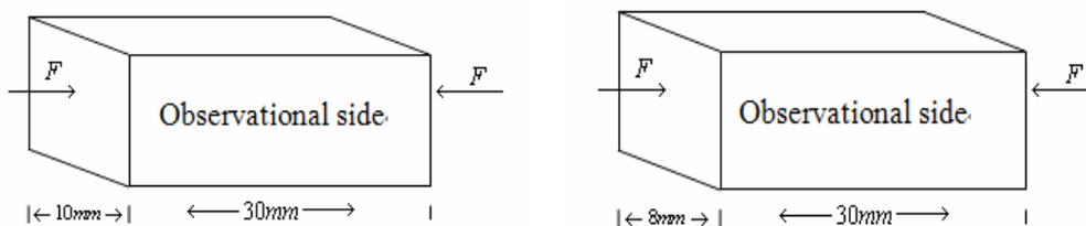
Figure-1 The sketch of loads exerted on 20steel and 45steel
