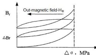
**Fig.1 Principle of magnetoelasticity effect**
