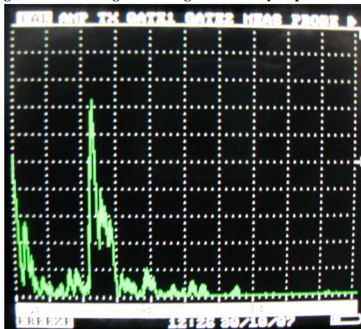
Fig.5 The waveform of ultrasonic inspection
