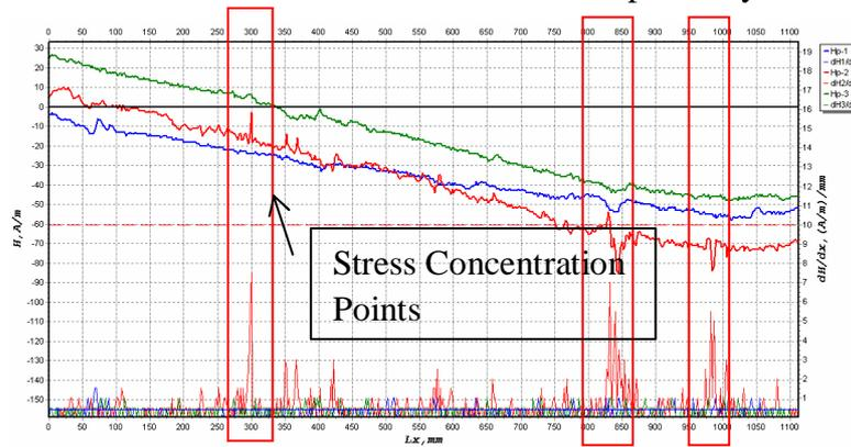
Fig.6 ZGa0054 straight tube magnetic memory inspection image
