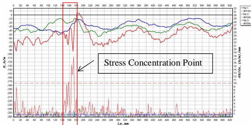
Fig.4 ZGa0002 straight tube magnetic memory inspection image
