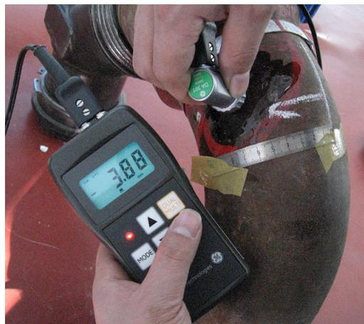
**Fig.8 The minimum wall thickness while ultrasonic thickness gauging**
