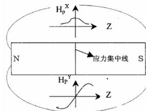
**Fig.2 Principle of magnetism memory inspection**
