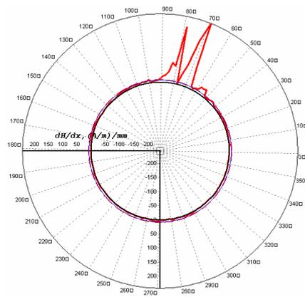
Fig.10 Magnetic memory inspection image of the bent pipe with pricker
