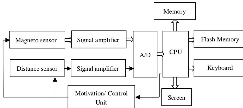
Fig.3 Principle of TSC series magnetism memory test devices
