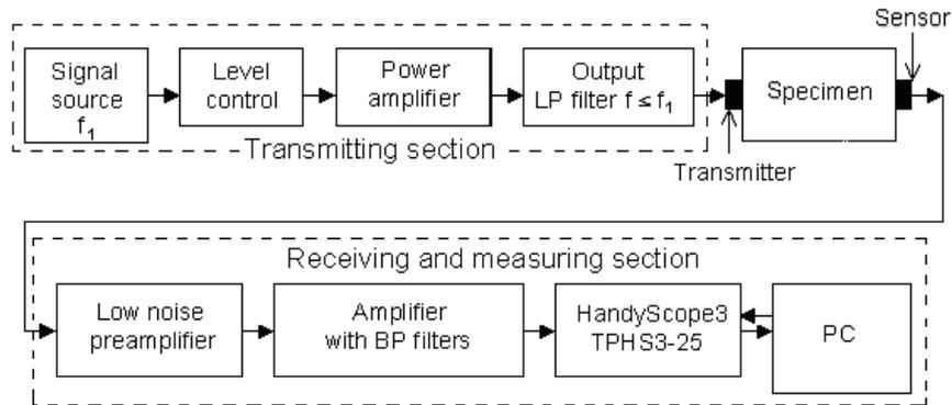
Fig. 2: Block diagram of the measuring apparatus
