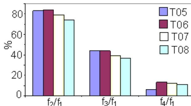
Fig. 6: Relative amplitude values - intact joists
