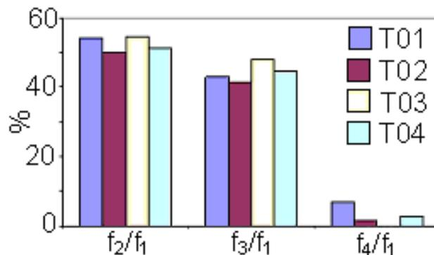
Fig. 5: Relative amplitude values - loaded joists
