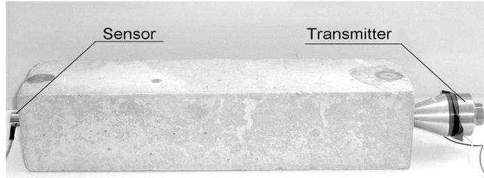
Fig. 3: Location of the transmitter and the sensor on the specimen under test
