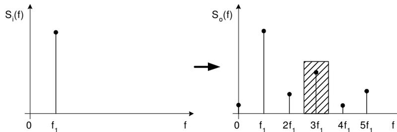
Fig. 1: Frequency spectrum of a non-linear medium response
