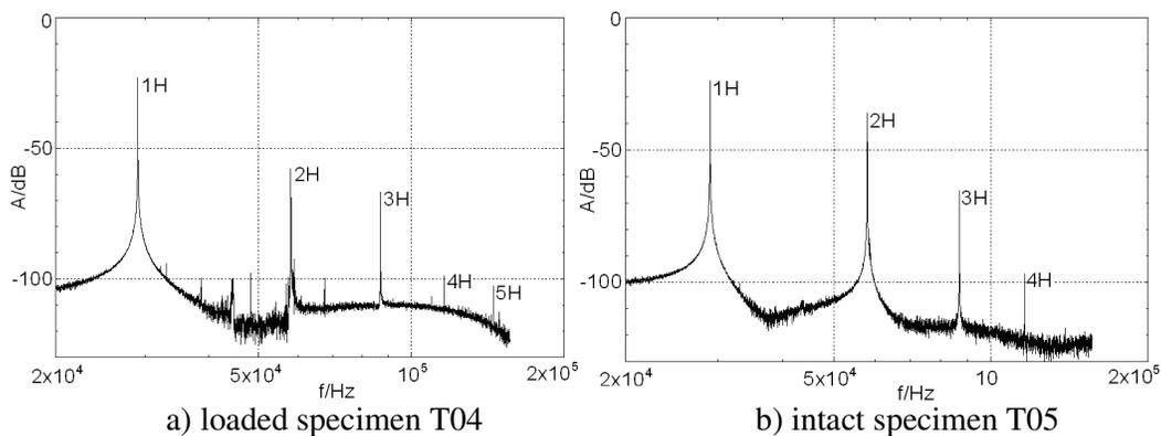
Fig. 4: Frequency spectra of concrete joists
