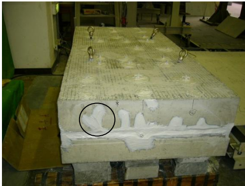
(a). The Cracks are sealed with epoxy resin.
