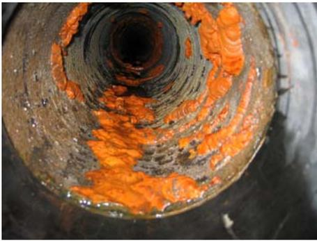
Internal tubercles are common in cast iron and steel water pipes. Scraping down to bare metal results in rusting that turns drinking water red for weeks; however, RFT is able to inspect cast-iron, ductile iron and steel pipelines through 25mm of scale, reducing the need for cleaning.
