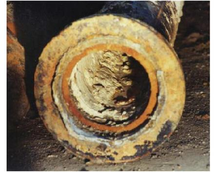
Fig-4a) and 4b) Showing internal scale in cast iron water pipe
