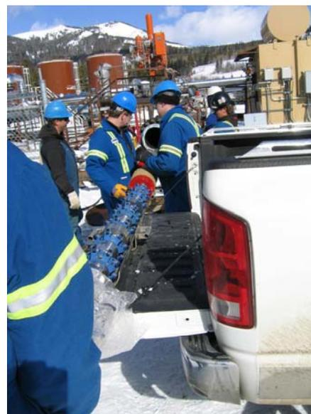
RFT requires a relatively low inspection speed; however, this limitation is far outweighed by its ability to inspect through scale deposits and liners.
