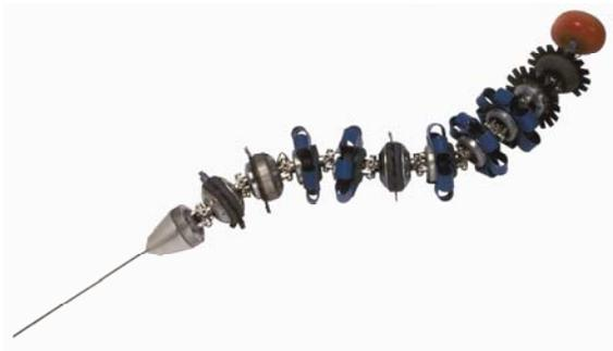
Fig-6a) (above) showing a tethered RFT tool
