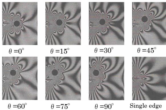
Fig.7 Example of photographs obtained by experiment (crack and circle hole,  $r =10\text{mm}$ ,  $F =2.45\text{kN}$ )
