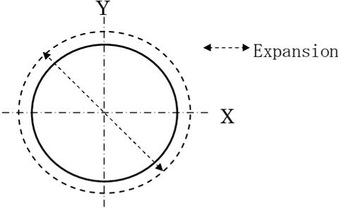
Fig. 2 Direction of stress for the specimen
