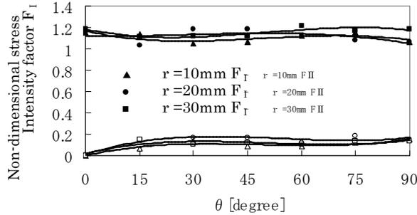
Fig.11 Relation between non-dimensional stress intensity factor F and angle  $\theta$  for inclusion
