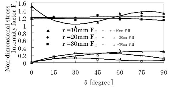
Fig.10 Relation between non-dimensional stress intensity factor F and angle  $\theta$  for circle-hole
