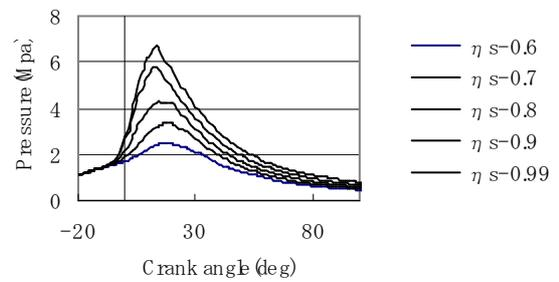
Fig.6 Comparison of pressure in cylinder
