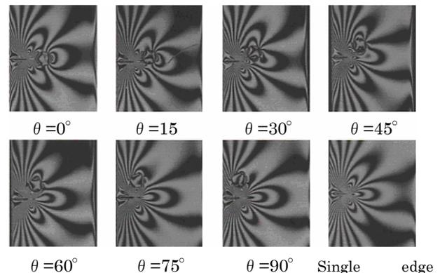
Fig.8 Example of photographs obtained by experiment (crack and circle inclusion,  $r =10\text{mm}$ ,  $F =2.45\text{kN}$ )
