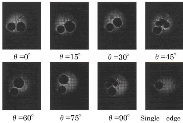
Fig.9 Caustic patterns of inclusion (2.45KN)
