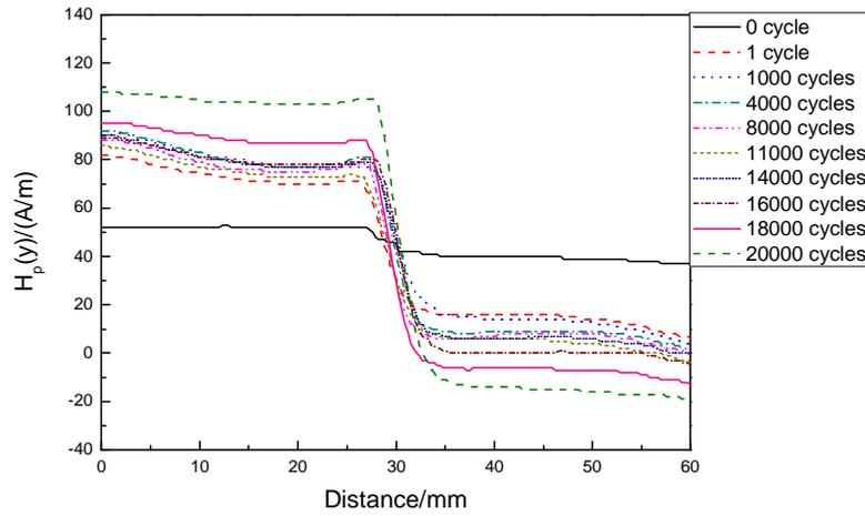
Figure 6. Magnetic signals of specimen 2 from line 5 at different cycles
