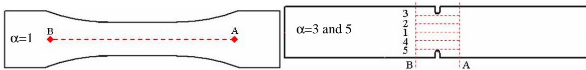
Figure 1. Testing paths of samples with different stress concentration factors
