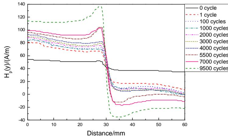
Figure 7. Magnetic signals of specimen 3 from line 5 at different cycles
