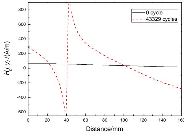
Figure 2. Magnetic signals of specimen 1 before loading and after fracture
