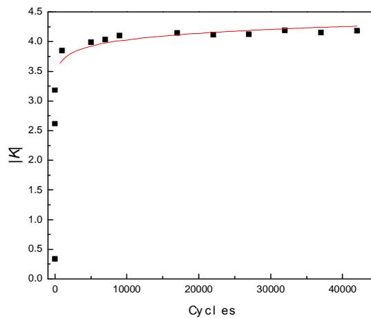
Figure 4. Gradient  $|k|$  of magnetic signals from line at different cycles of specimen 1
