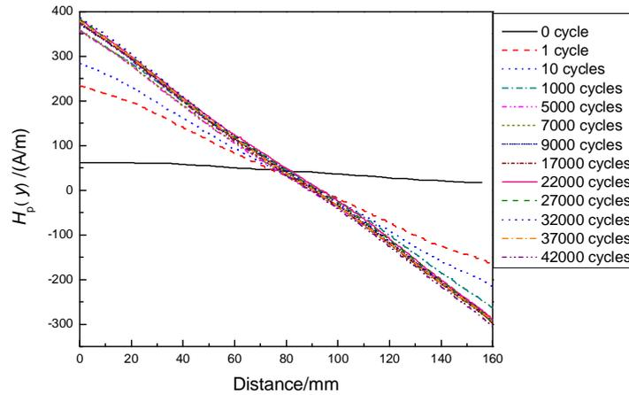
Figure 3. Magnetic signals from measured line at different fatigue cycles of specimen 1
