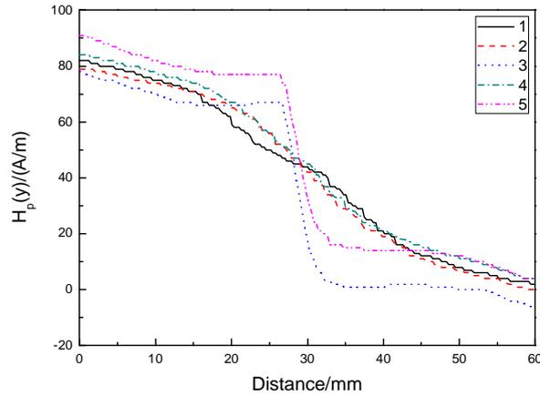
Figure 5. Magnetic signals of specimen 2 from different measured lines at 1000 cycles
