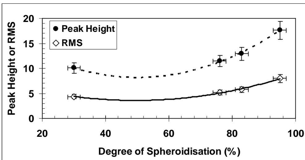
**Figure 3.** Degree of spheroidisation and MBN parameter correlation
