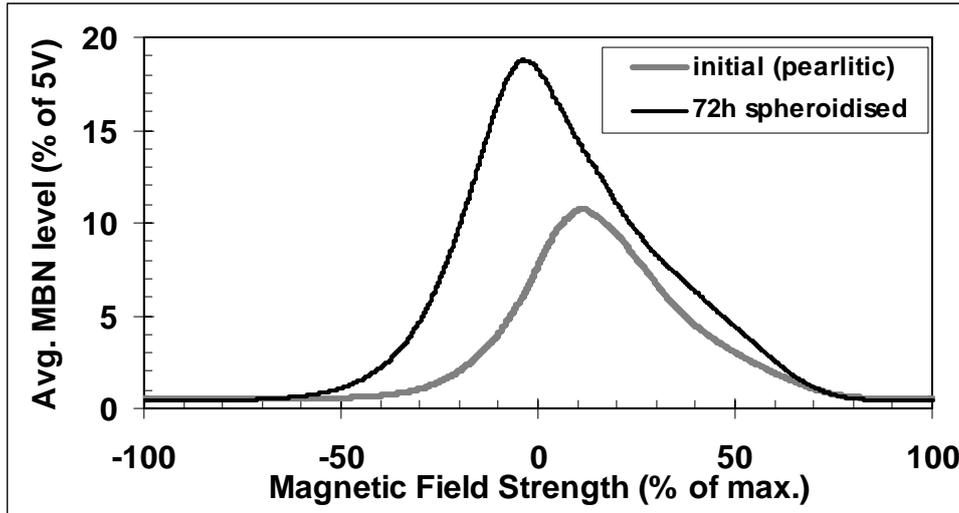
**Figure 2.** MBN profiles of the specimens
