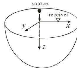
Fig. 1 Coordinates of a half-space with a point source applied at the origin.
