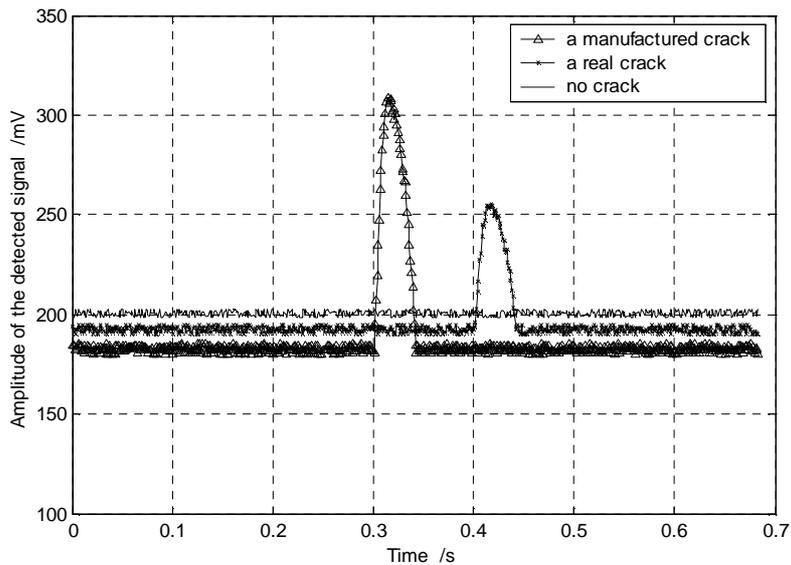
Fig.7 the Inducted Voltage Amplitude-time Response Curve of Pick up Coil
