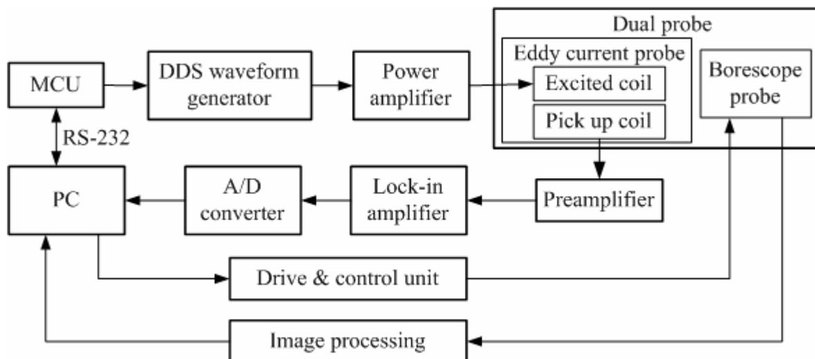
Fig.5 the NDT System Block Diagram Using Borescope and Eddy Current Dual Probe
