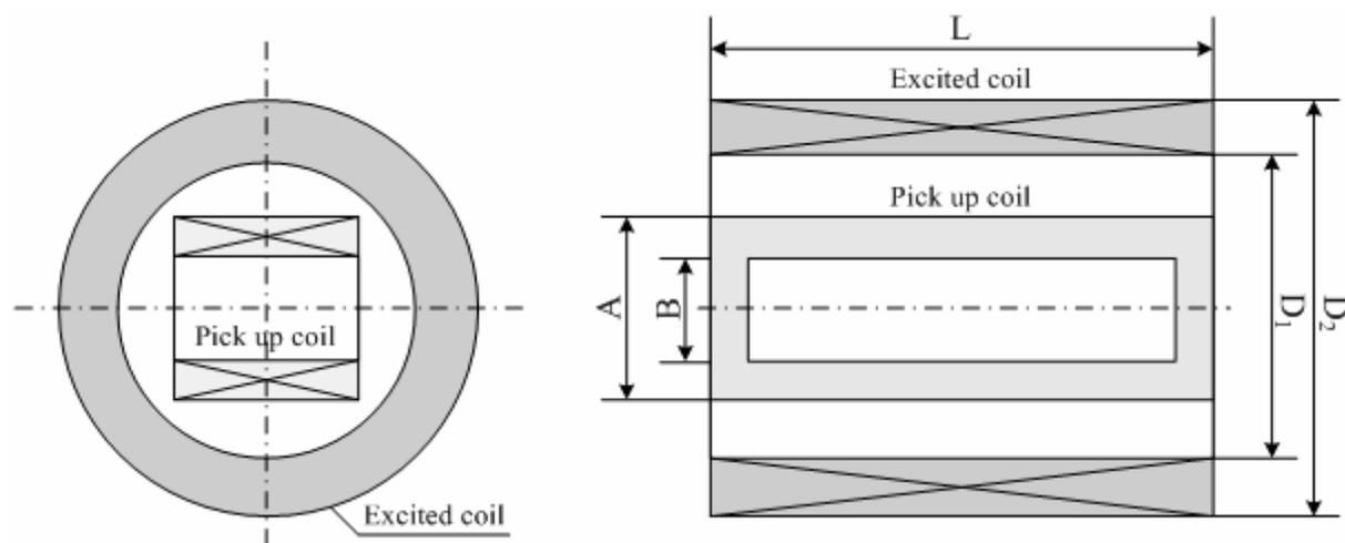
(a) the Cutaway Vertical the Axes of Excited Coil      (b) the Cutaway Vertical the Axes of Pick Up Coil
