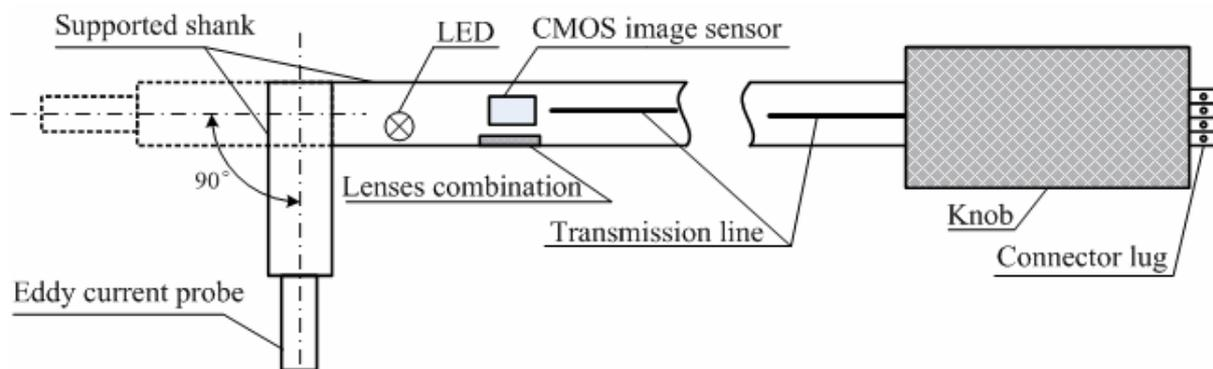
Fig.3 the Schematic Structure of the Borescope and Eddy Current Dual Probe
