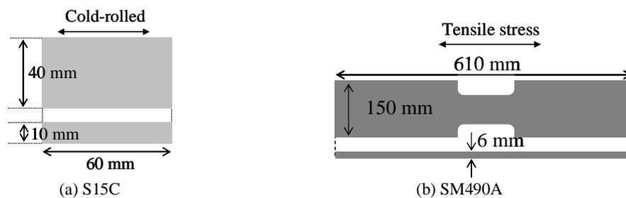
Fig. 1 The dimension of the plates.
