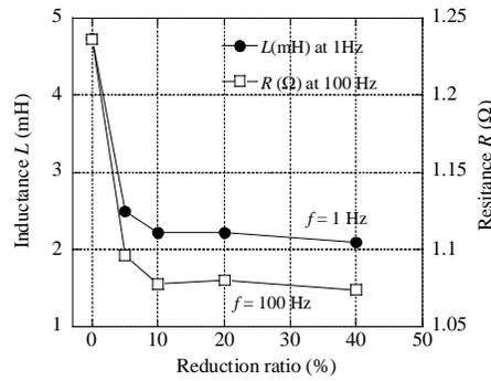
Fig. 6 Relation between impedance and the reduction ratio for S15C steel.
