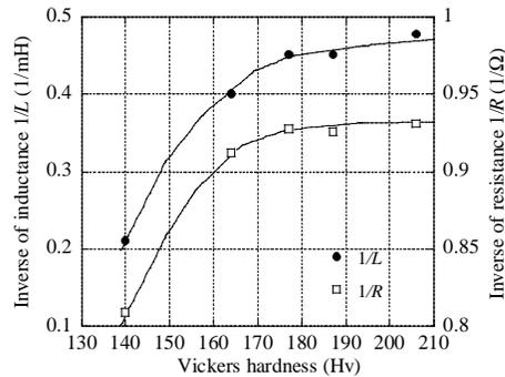
Fig. 7 Relation between impedance and Vickers hardness for S15C steel.
