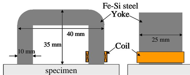
Fig. 2 The dimension and the configuration of the single-yoke.
