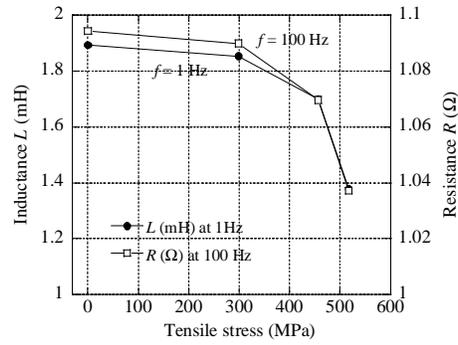
Fig. 8 Tensile stress dependence of impedance for SM490A steel.
