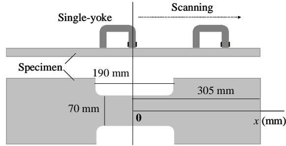
Fig. 3 Explanation for scanning the single-yoke over the SM490A plates.
