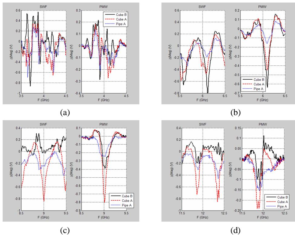
Figure 4. Normalised differential spectra for PMW and SFW with respect to centre frequency set at: (a) 4GHz; (b) 6GHz; (c) 9GHz; (d) 12GHz
