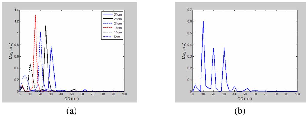
Figure 2. Spectrum analysis for OD against object positions: (a) single object; (b) multiple objects
