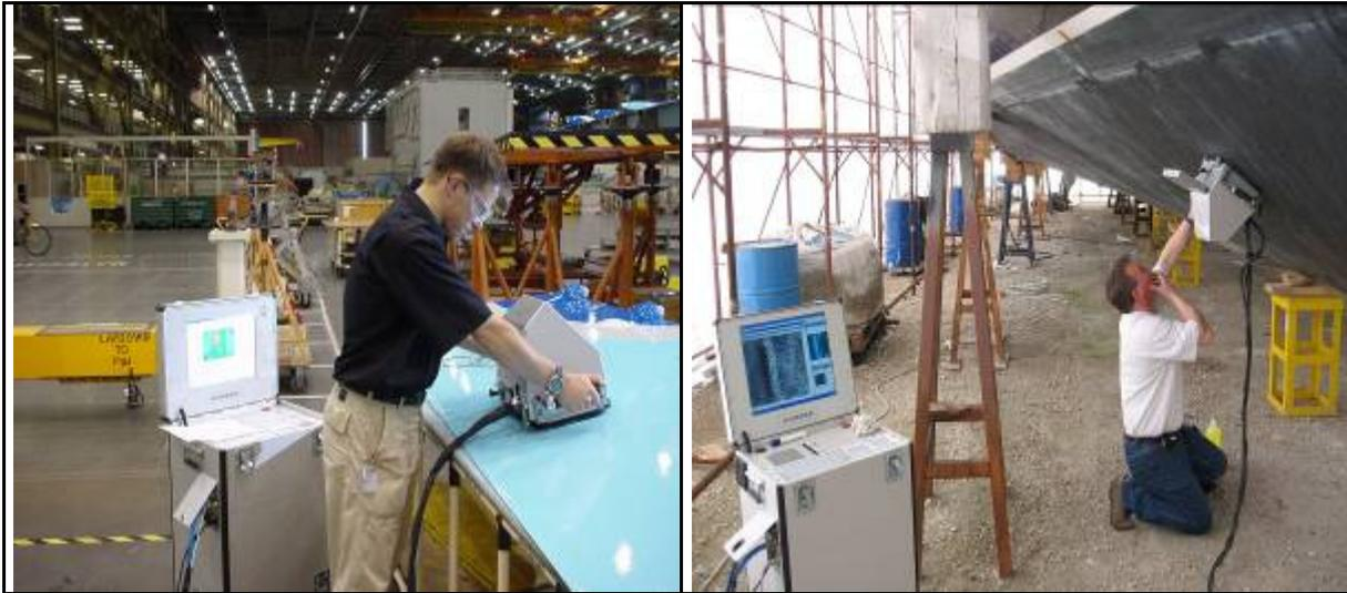
Fig. 7: Portable shearography system for field inspection of composite materials      Fig. 7: Portable shearography system in situ on a boat structure
