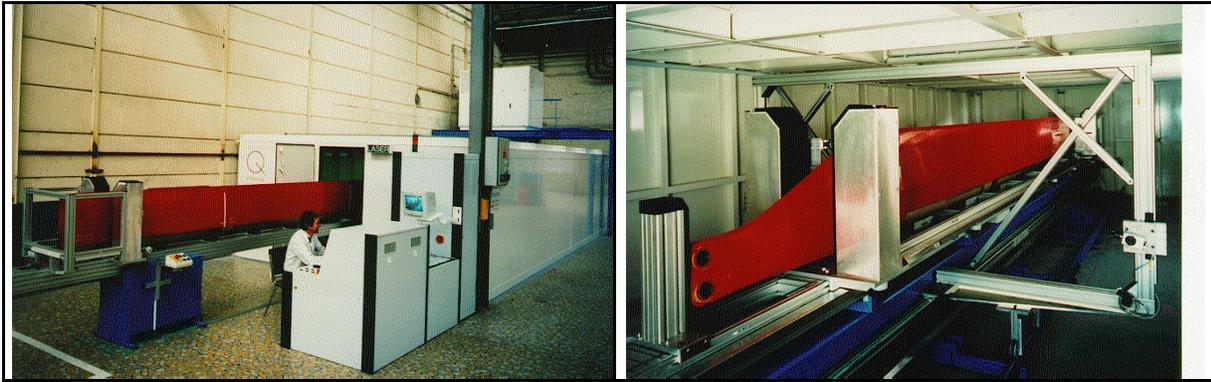
Fig.1: Helicopter rotorblade inspection system Fig.2: View inside the vacuum chamber with rotorblade in testing position
