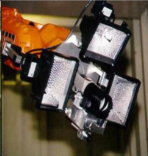
Fig.4: Sensor, illumination optic, thermal loading defect marking system on the tip of the robot.
