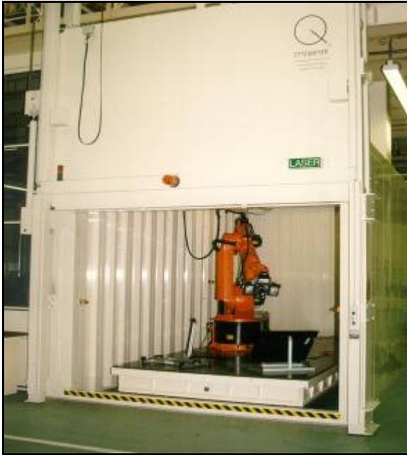
Fig.3: 6-axis industry robot in automatic inspection system of thermal protection parts.
