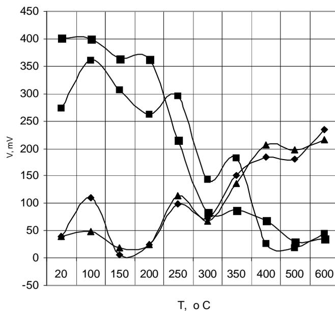
Fig.4. Dependence of BNP upon the tempering temperature of hard quenched medium carbon steel before (curves 1 and 2) and after abrasive treatment (curves 2 and 4) at longitudinal (curves 1 and 3) and transversal (curves 2 and 4) magnetizing field directions.
