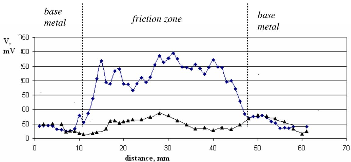
Fig.3. Spatial distribution of BN parameter along the specimen from spring steel after its abrasive treatment by the ceramic rider
