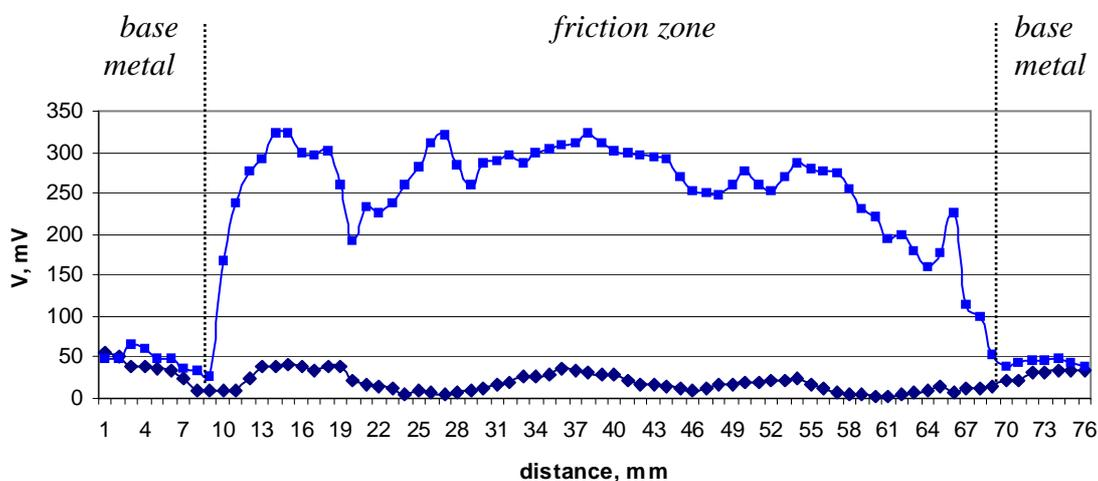
Fig.2. Spatial distribution of BN parameter along the specimen from tool steel after its abrasive treatment by the copper rider
