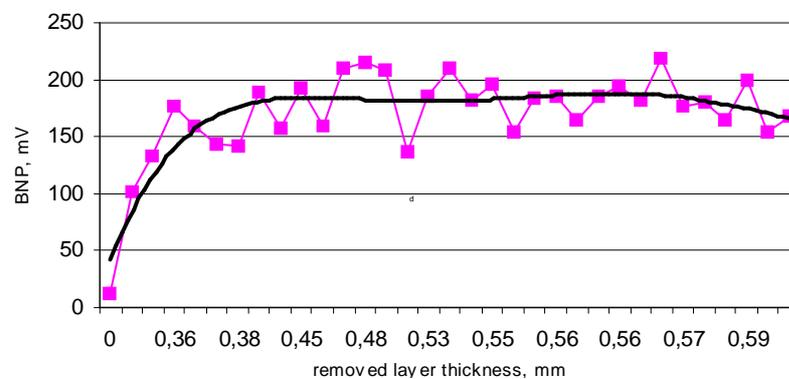
Fig.1. The dependence of Barkhausen Noise parameter via the thickness of the layer removed by grinding.
