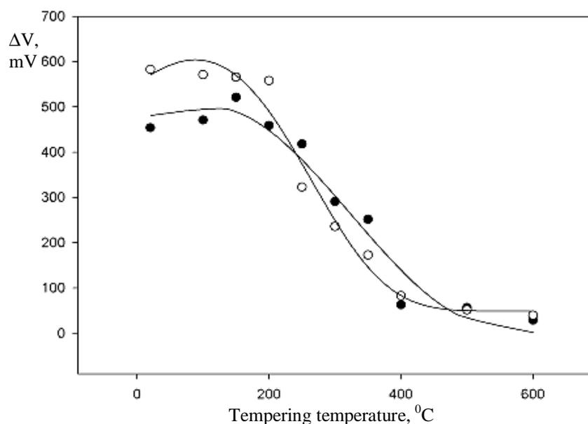
Fig. 5. The differences, curves 1 and 2, between respectively curves 1 and 3 and also 2 and 4 in the fig.4, which show the real influence of tempering effect on the abrasively treated surface.
