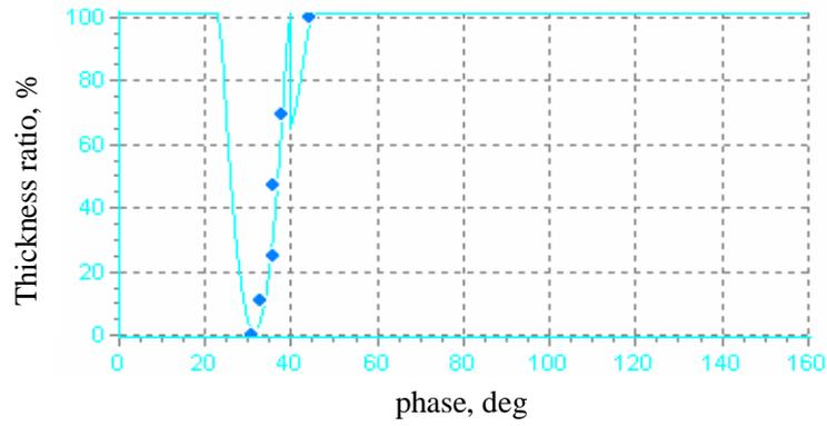
**Fig.4 calibration curve of coating thickness vs phase**
