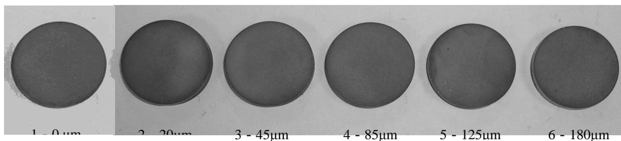
Fig.1 Specimens with various thickness brush-electroplated nickel coatings
