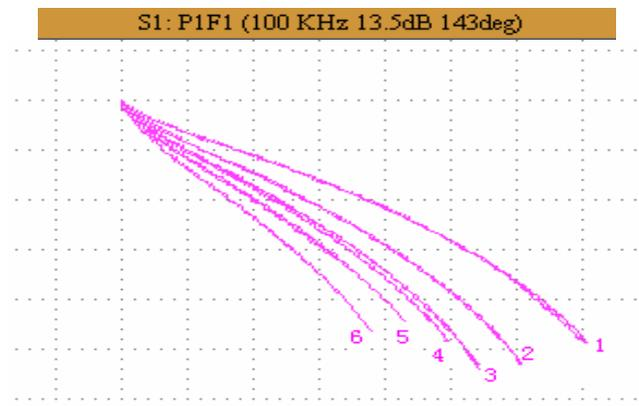
**Fig.2 Impedance curves of the six samples at frequency 100KHz**
