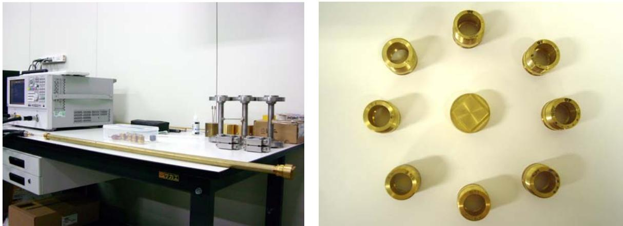
(a) The microwave instrument for transmitting and receiving microwave signals
