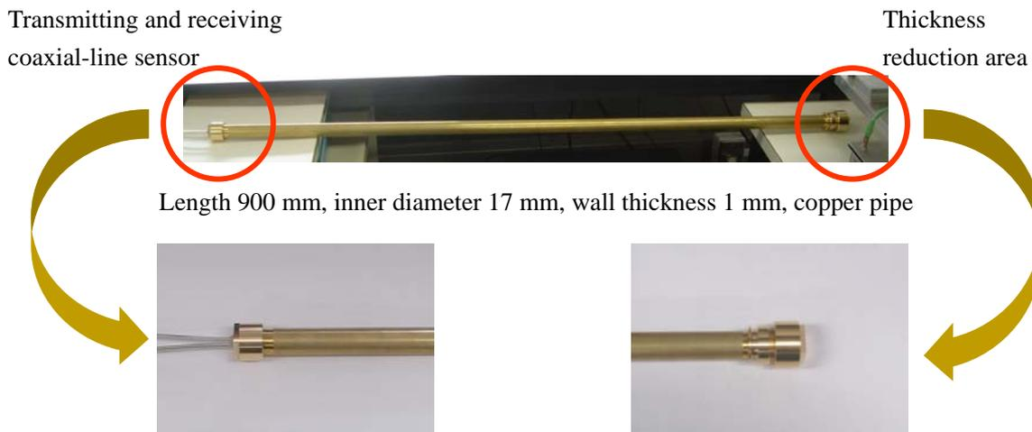
**Fig.2** Sensor and the cap connected at the terminal of the experimental specimen
