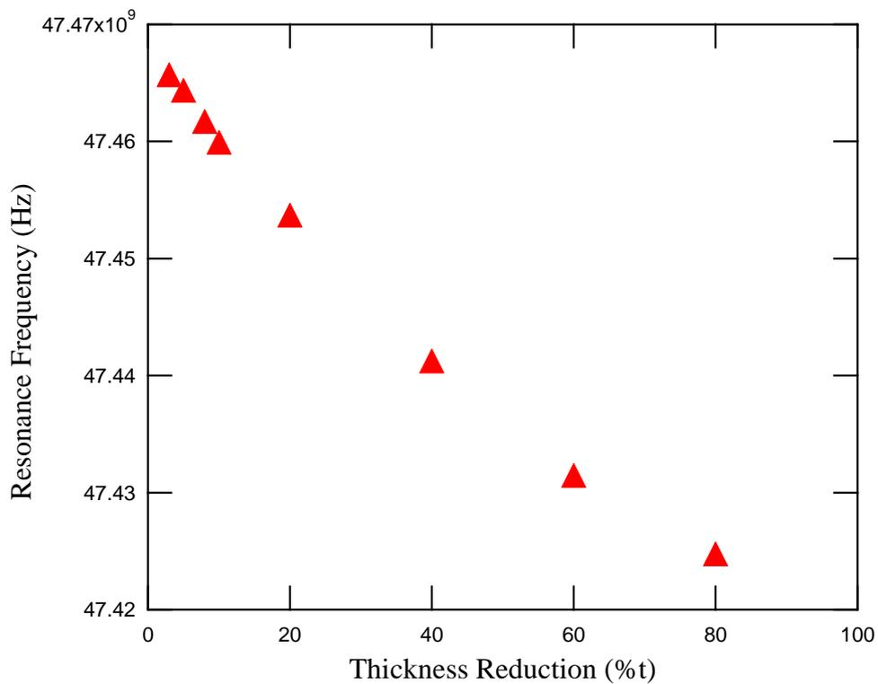
**Fig.4** Relationship of resonance frequency and thickness reduction
