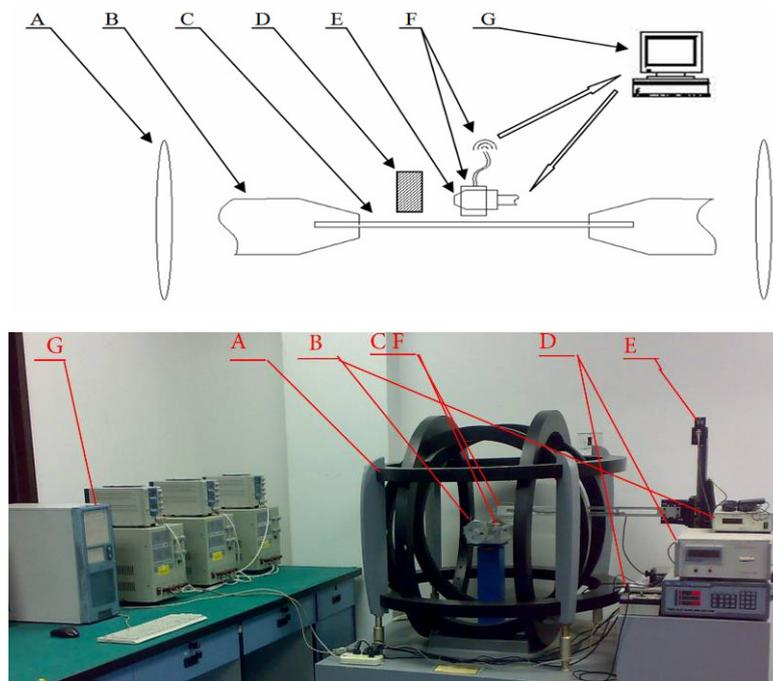
Fig.1 Experiment System ( A: 3D Helmholtz Coil; B: Portable Tensile Means; C:Specimens; D: Flux Gate Magnetometer and Tesla Magnetometer; E: 3D Displacement Controller, F: Wireless Micro-magnetic Detector and the GMR Sensor, G:Computer)
