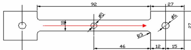
Fig.2 Specimen dimensions and scanning line
