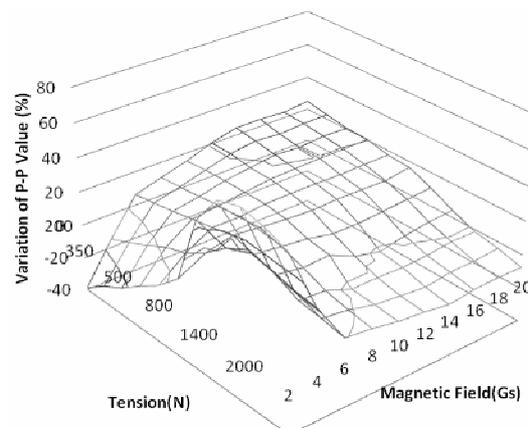
Fig.8 Effect of magnetic field in generation of MMM signals
