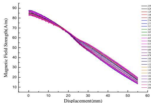
Fig.4 MMM signal of each tensile stress under geomagnetic field
