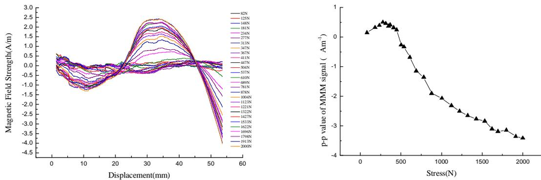
a. the magnetic distortion caused by stress concentration under geomagnetic field
