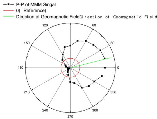
Fig.6 The P-P value of MMM signal changes with the direction of geomagnetic field
