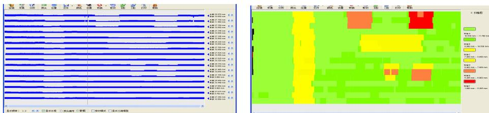
Figure 2 B-type and C-type display of thickness
