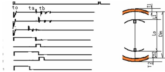
Figure 1 Principle of inspecting pipe thickness and diameter and typical wave forms of broad-band ultrasonic
