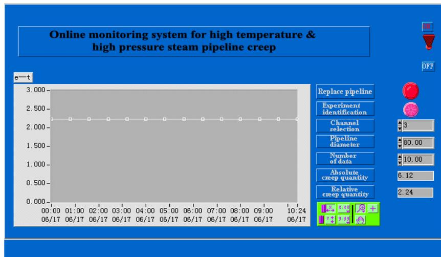
Fig.6 When the relative creep deformation quantity reaches 2%, the system will sound the alarm and suggest replacing the pipeline.
