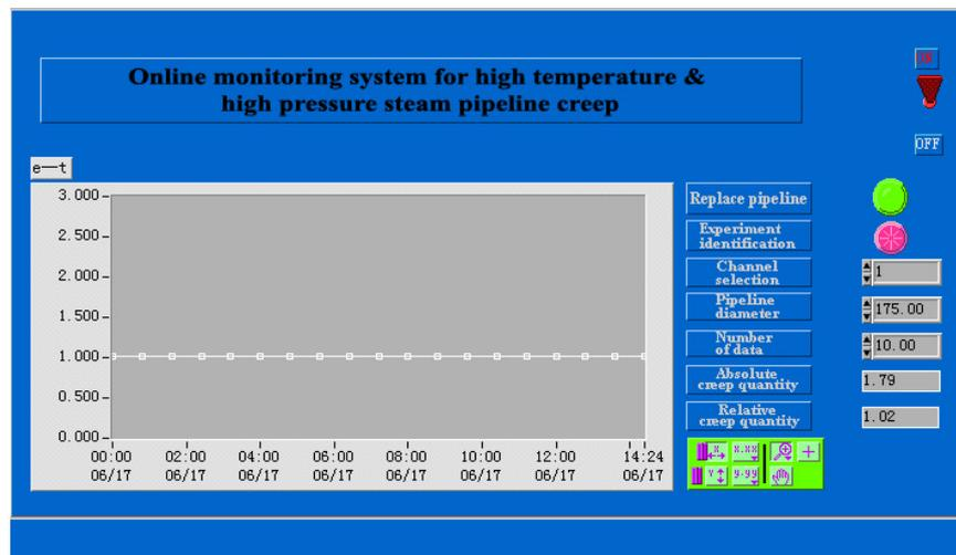
Fig.5 When the relative creep deformation quantity reaches 1%, the system will sound the alarm and suggest an experiment identification.
