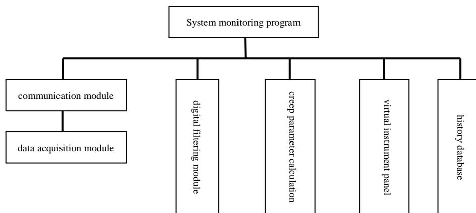
Fig.4 The block diagram for the system software structure
