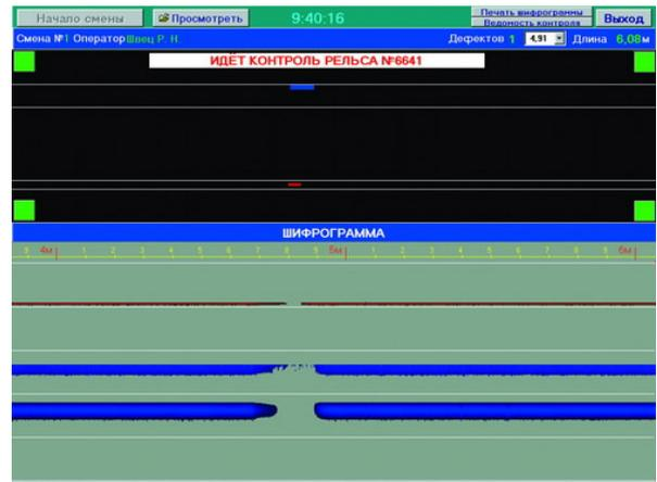
Fig. 4. Internal rails' defects and their defectograms
