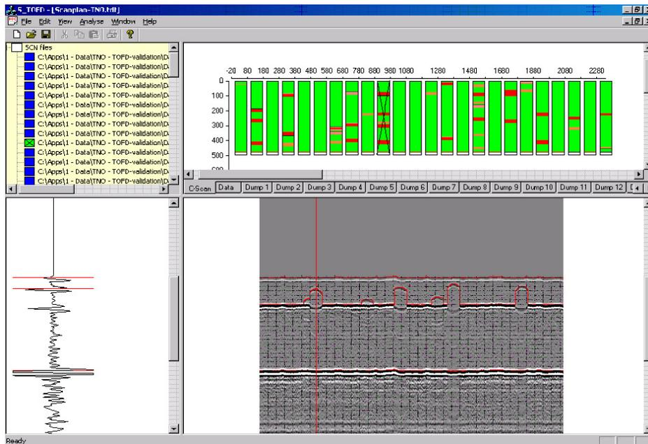
**Figure 7** Simulated TOFD B-scan image imported into TOFD analysis software for interpretation..
