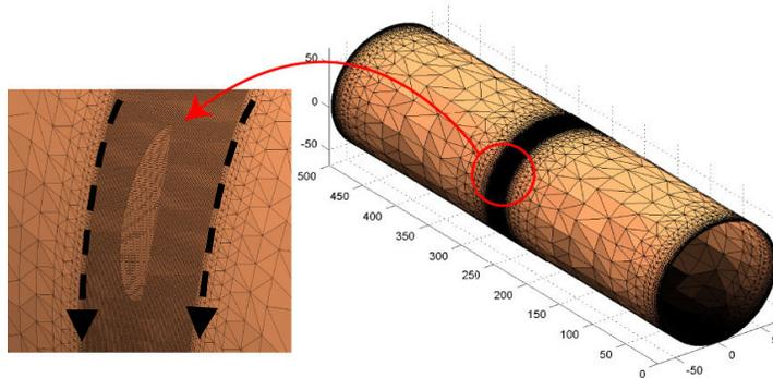
**Figure 4** Mesh describing the inner surface of a simulated pipe with a fatigue crack near the root of a circumferential weld. The dashed arrows indicate the TOFD scanning direction.
