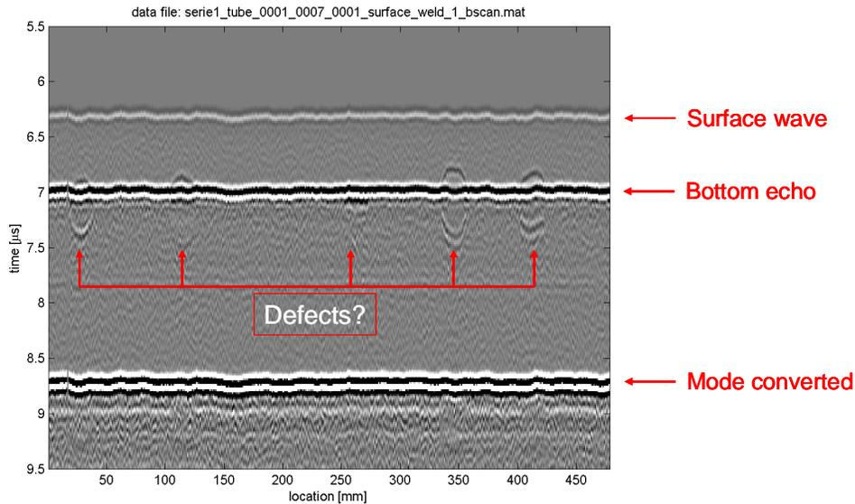
**Figure 6** Simulated TOFD B-scan image for a number of defects, i.e. weld root fatigue cracks.
