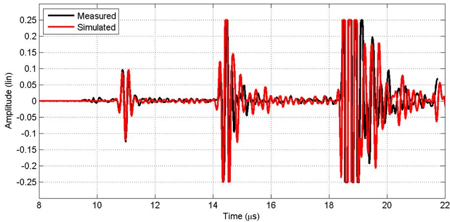
**Figure 2** Validation of modeling ultrasonic TOFD inspection comparing measured and simulated A-scans. Measurement setup: probe distance 50 mm, probe angle 60°, frequency 5 MHz and crystal diameter 3 mm.
