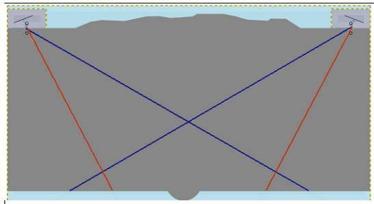
**Figure 5** Simulation set-up of the TOFD modeling
