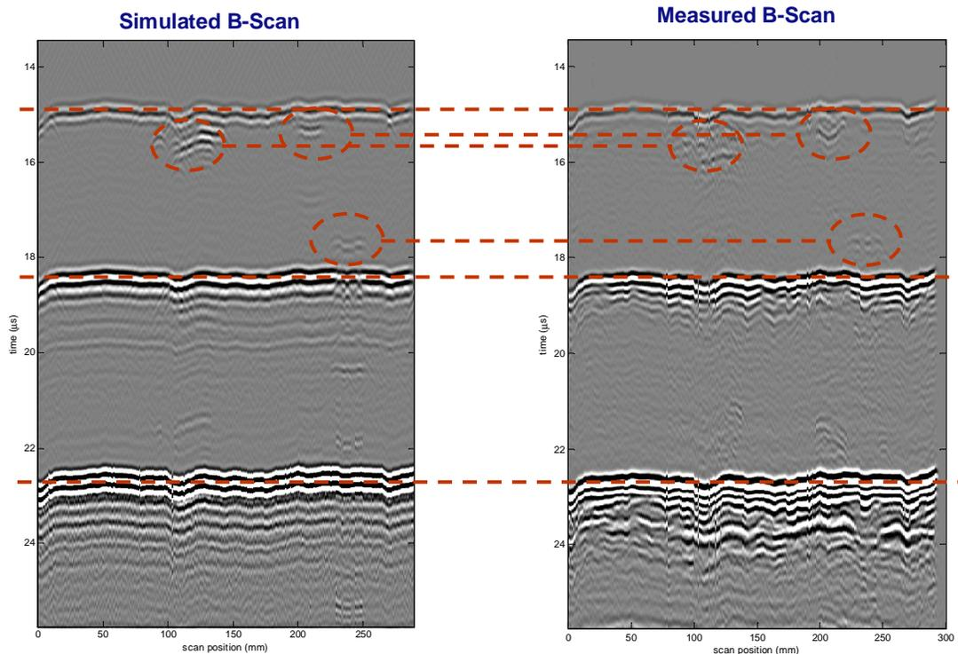
**Figure 3** Validation of modeling ultrasonic TOFD inspection by comparing measured and simulated B-scans. From left to right three defects can be discerned: around scan position 125 several gas inclusions, at position 220 a slag inclusion, and a root crack around position 240.
