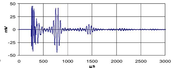
Figure 3: The propagation of longitudinal wave mode in an insulated wire at 20 kHz
