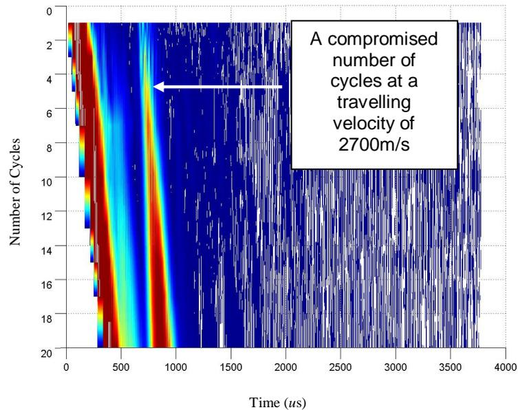
Figure 4: Experimental results for insulated wire at 60 kHz
