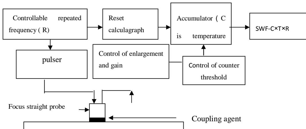
Figure 2 Principle chart adopting focus straight probe
