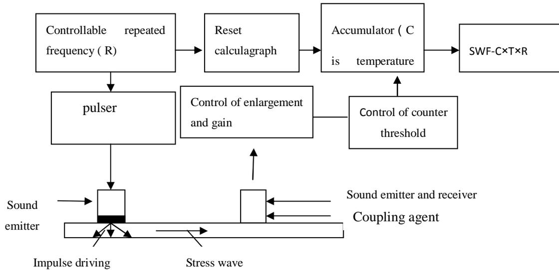
Figure 1 Principle chart of Ultrasonic Testing
