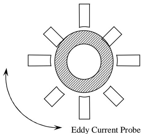
Figure5 Eddy current magnetic leakage probe array
