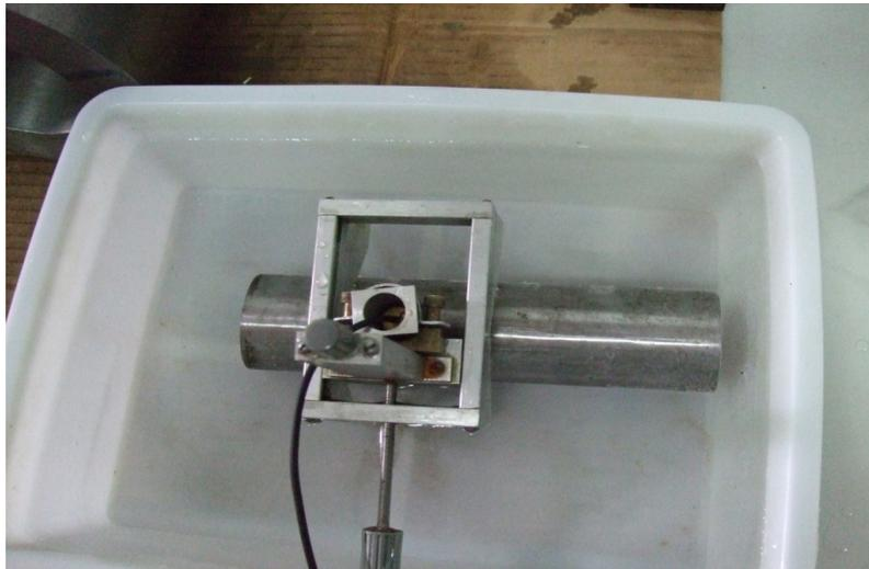
Figure 3 Sensor composite material tube and mechanism experimental apparatus
