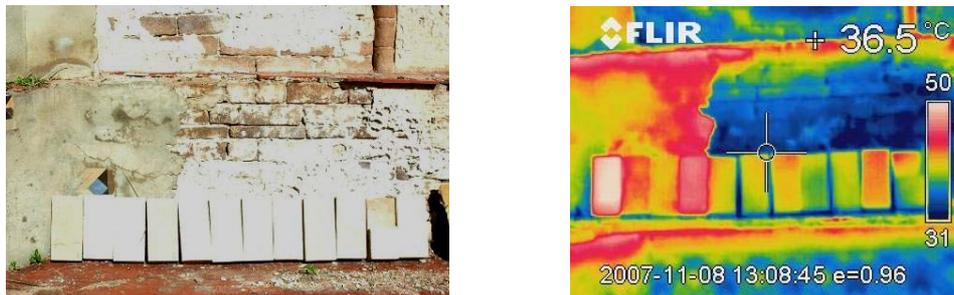
Fig 5. Comparison of mortar probes prepared at the Laboratory with mortar
