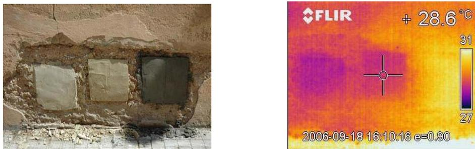
Fig. 6. Probes made on site (left), later analysed by IRT images (right) for its identification.
