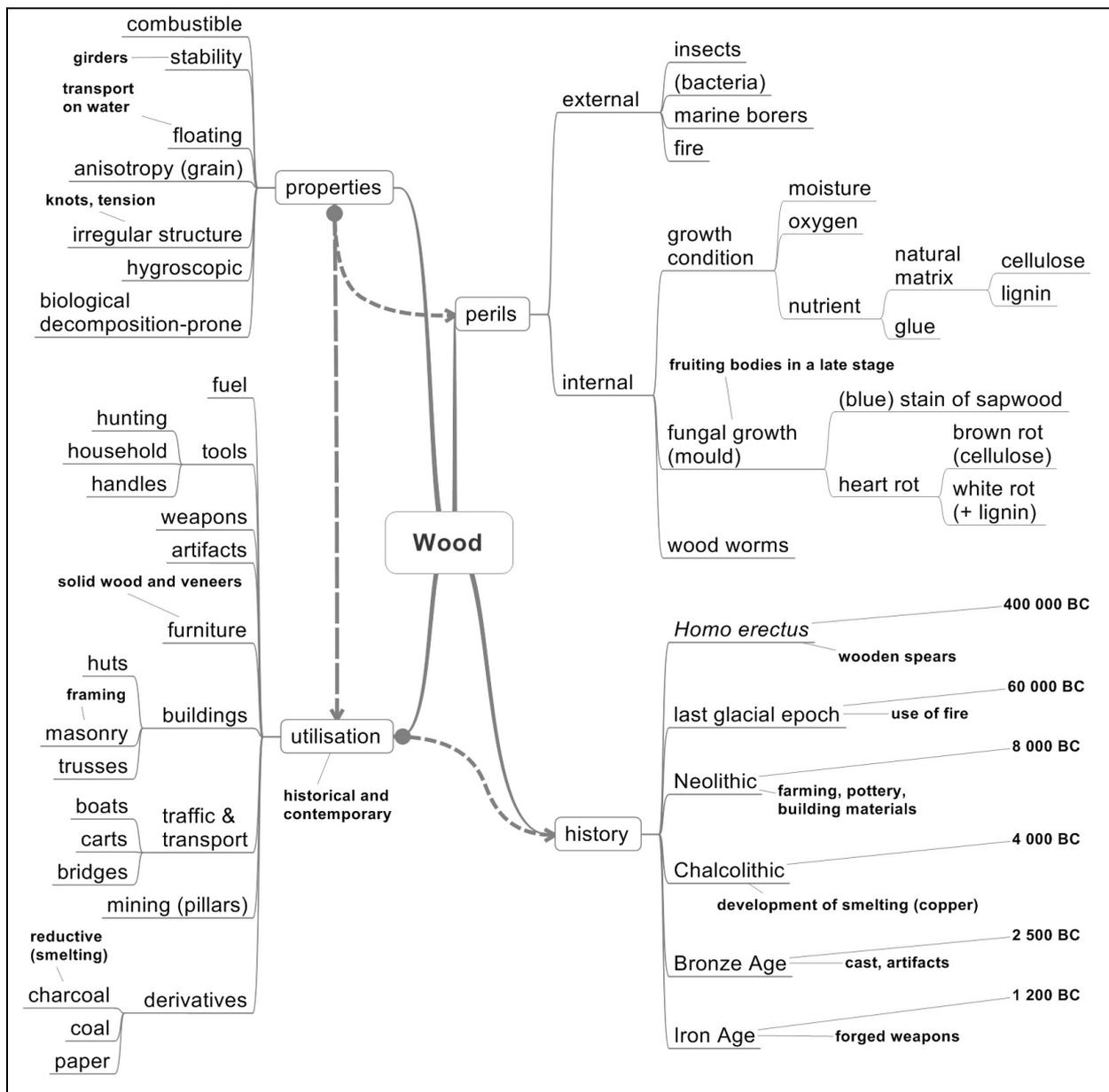
Figure 1. Properties of wood making its central role as the timeless material of mankind
