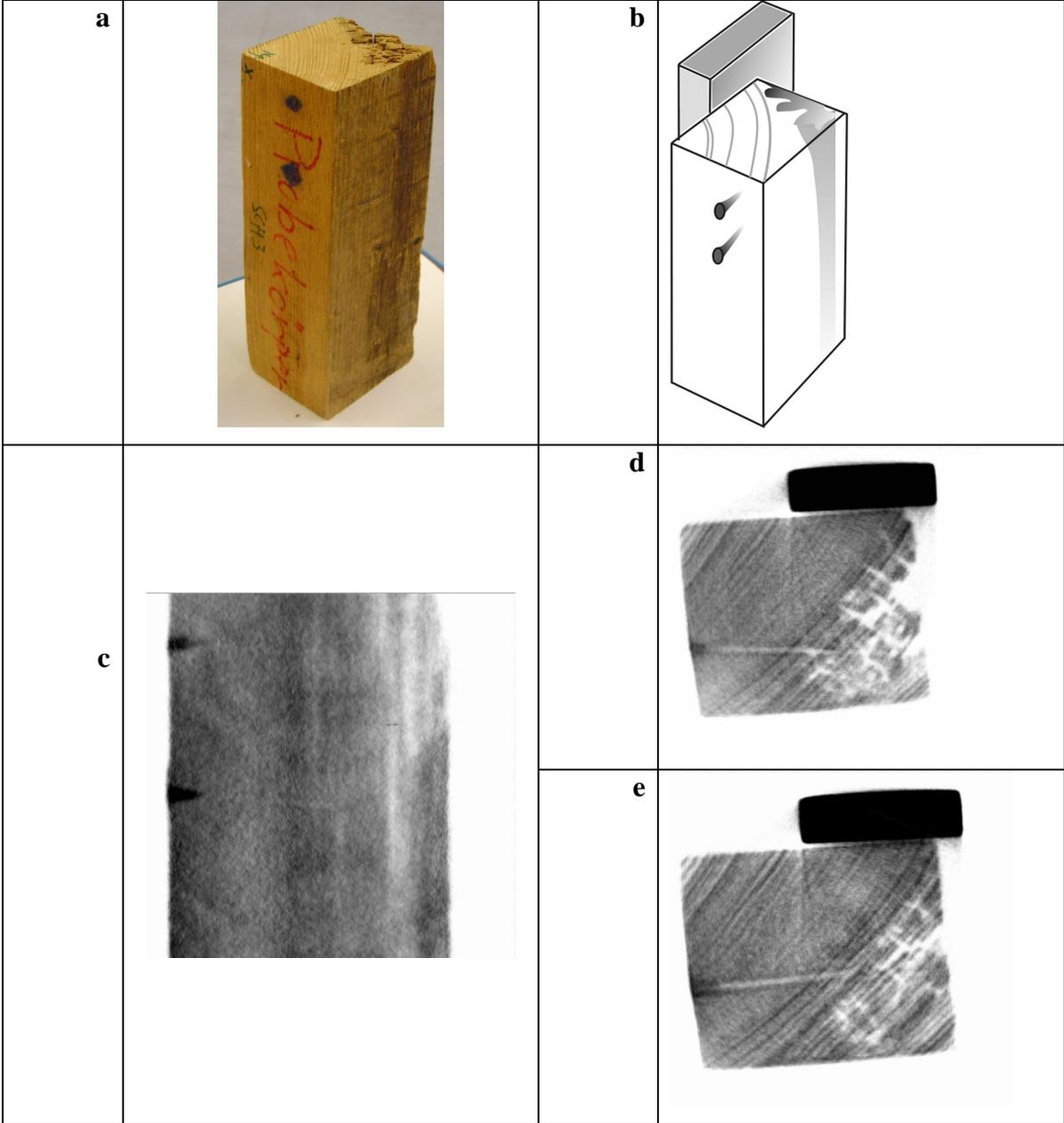
**Figure 2:** Tomography of a square shaped timber with flaws and inclusions
