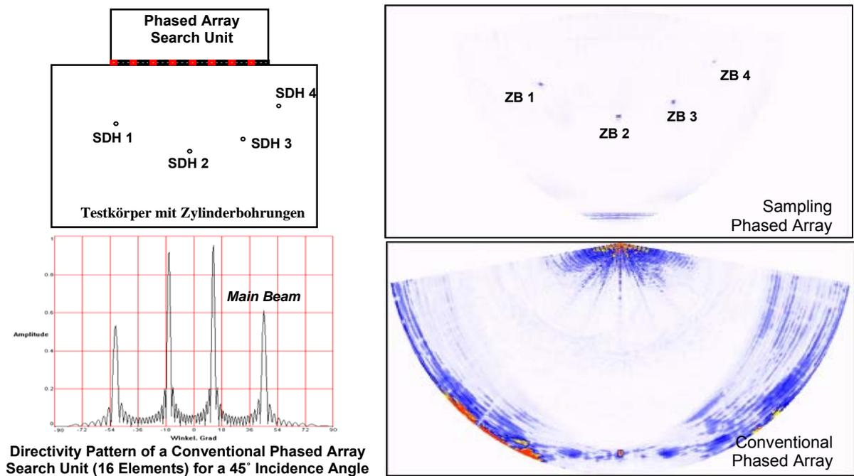
Figure 8. Image Reconstruction with Distributed Aperture
