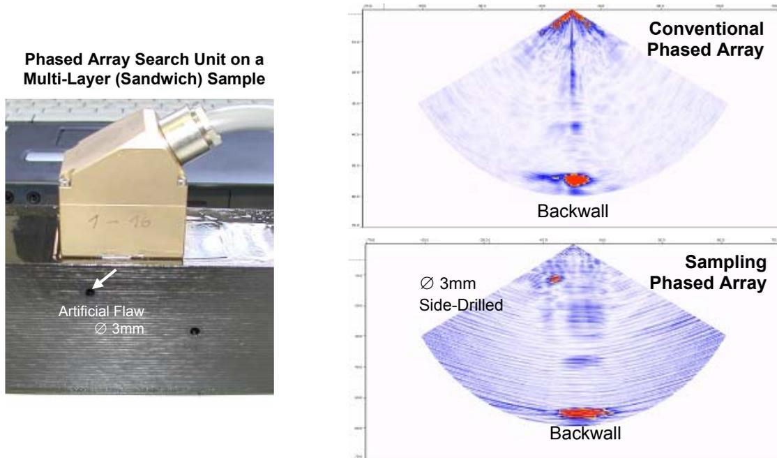
Figure 10. Test Results from a Multi-Layer Carbon-Fiber Sample using PA and SPA Techniques
