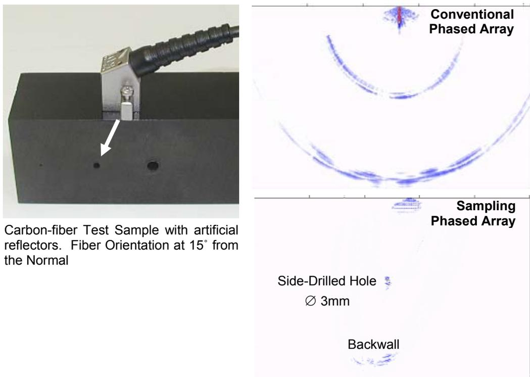
Figure 9. Test results from a monolithic carbon-fiber sample using conventional PA and SPA
