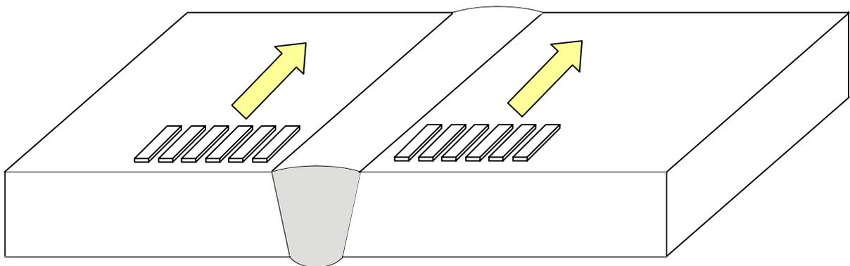
Figure 12. Transducer Array for Detecting and Evaluating Longitudinally Oriented Flaws; the Search Unit is Moved Parallel to the Weld
