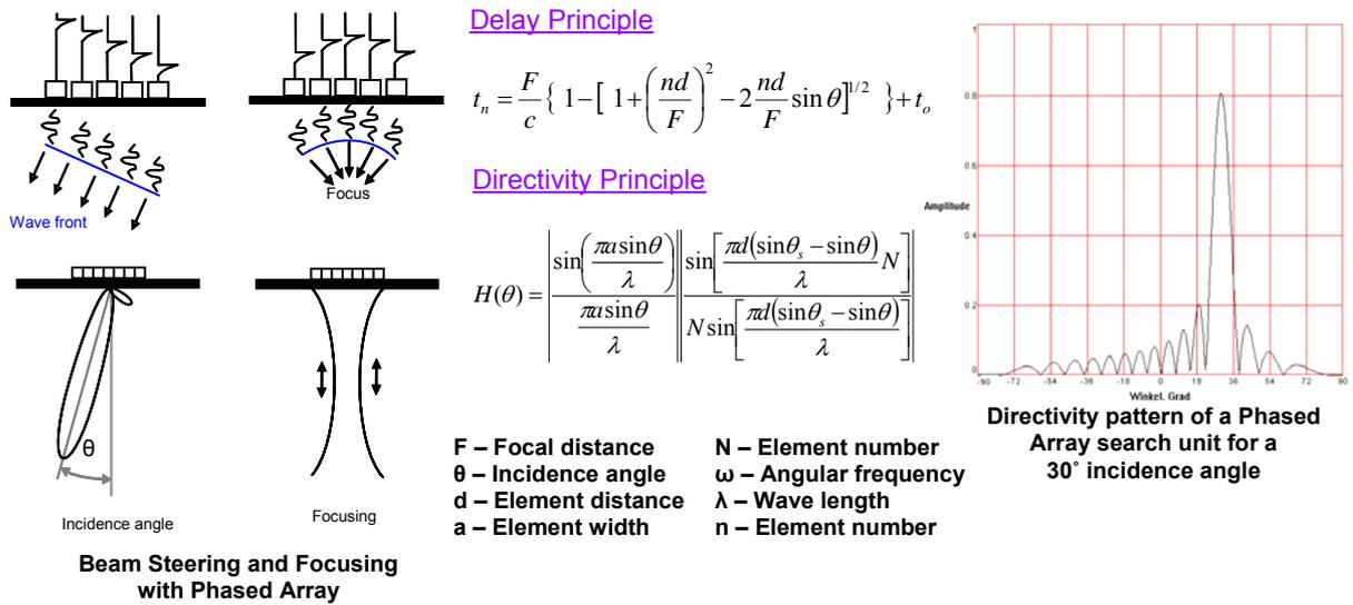
Figure 3. Data acquisition and Processing for conventional Phased Array
