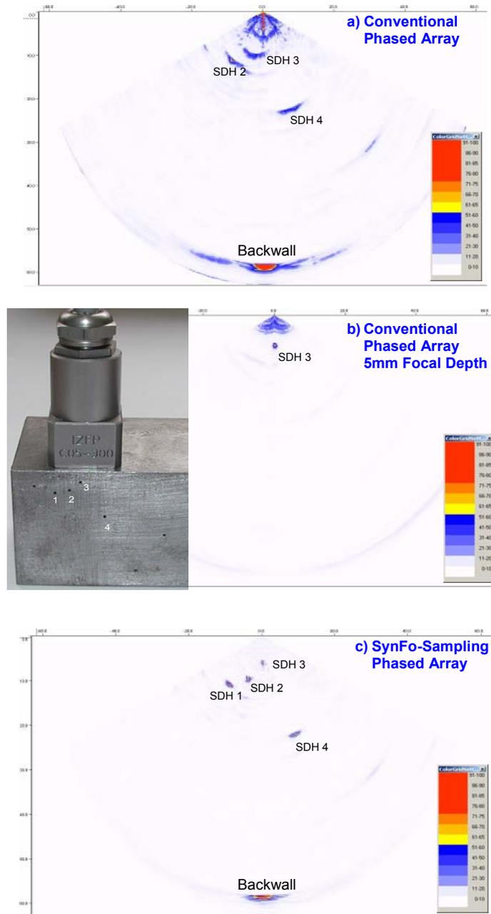
Figure 5. Near-field Measurements with conventional PA and SPA
