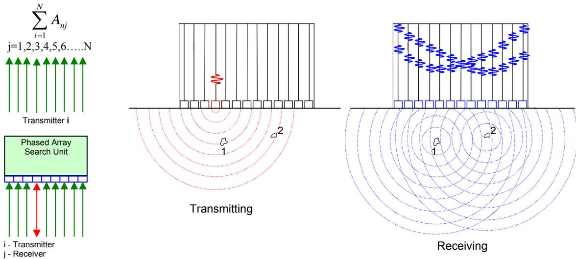
Figure 4. Data acquisition and Processing for Sampling Phased Array
