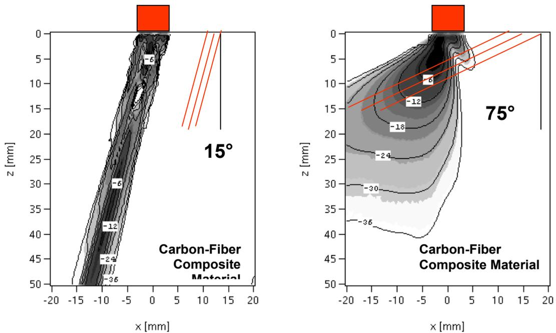
Figure 10. Sound Field Distribution of a 2 MHz Straight Beam Transducer on a Carbon-Fiber Composite Material (anisotropic) Test Sample
