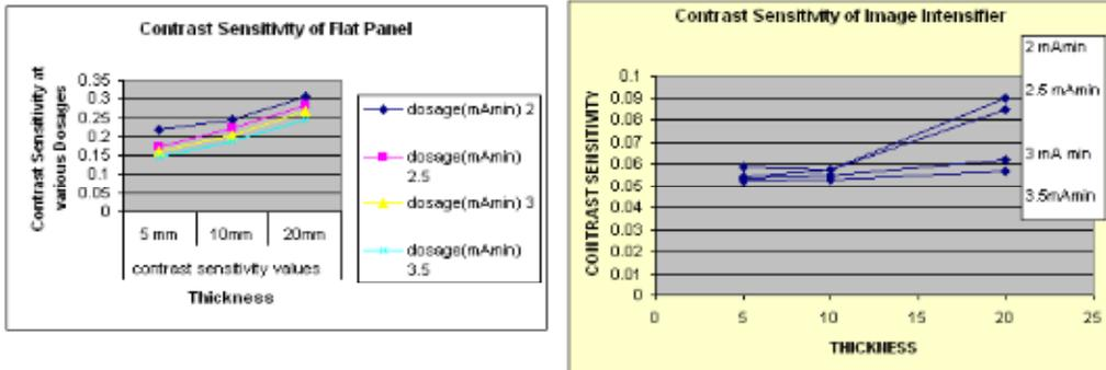
Fig. (3). Contrast Sensitivity Comparison between Image Intensifiers and Flat Panels
