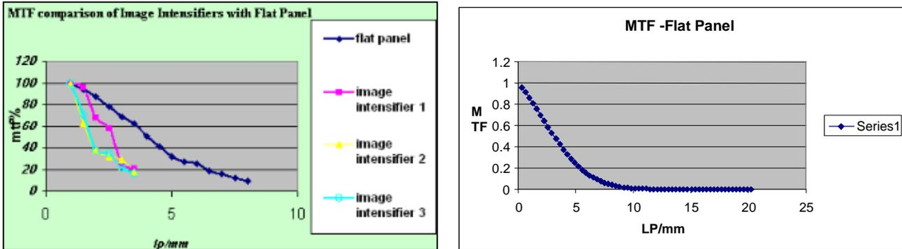
Fig. (1). MTF comparison between flat panel and Image Intensifiers
