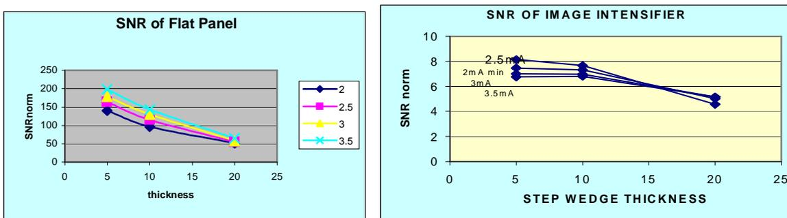
Fig. (4). SNR comparison between Digital Flat Panel and Image Intensifier.
