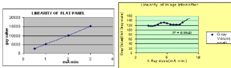
Fig.(2).Linearity Comparison between Flat Panel and Image Intensifier
