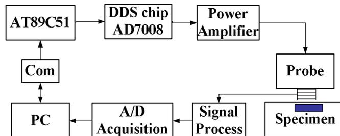
Figure 2. The schematic diagram of the experimental system
