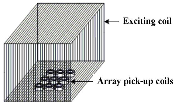
Figure 4. The schematic diagram of array PEC probe
