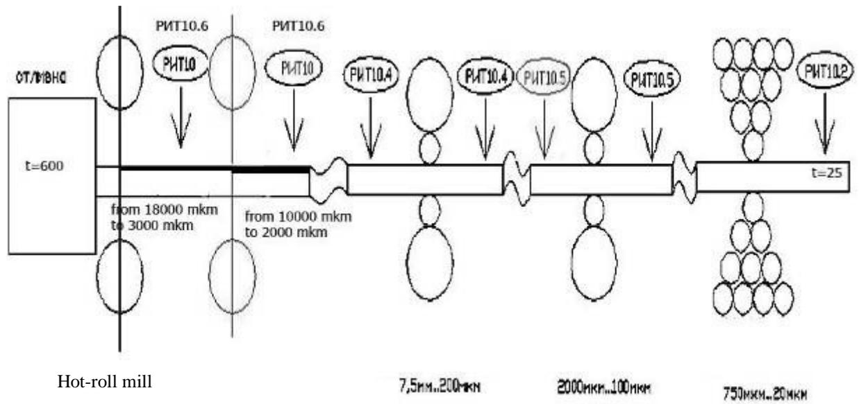
**Fig.1. Arrangement of Thickness Gauges on Roll Mills in Nickel Band Production**
