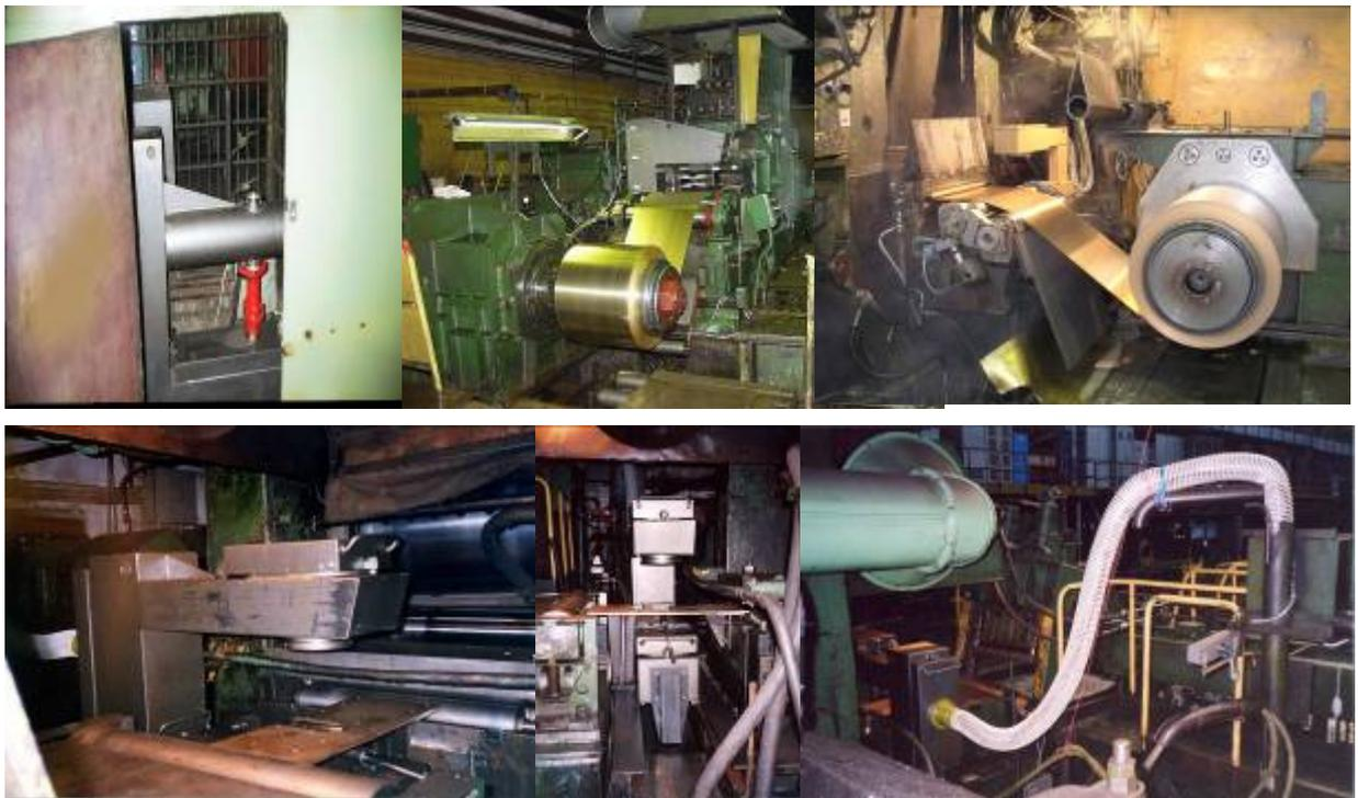
**Fig.2. RIT10 X-ray Thickness Gages at the Rolling Shop**
