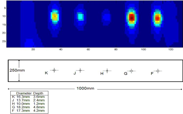
**Figure 3. Normalized signals while scanning over a plate with 5 emulated conical defects.**
