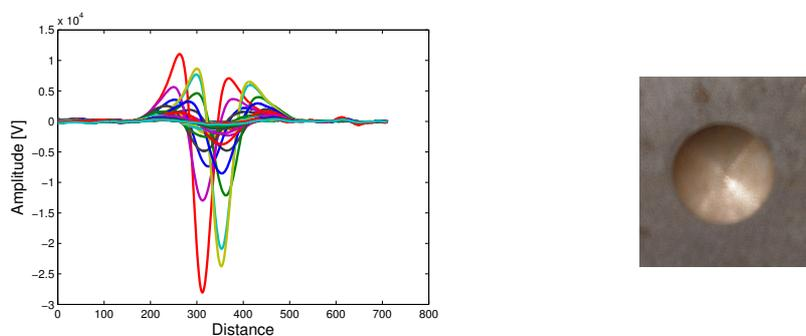
**Figure 2.a) Signals obtained over conical defect, b) Defect conical with diameter 17.3mm and depth 4.8mm**
