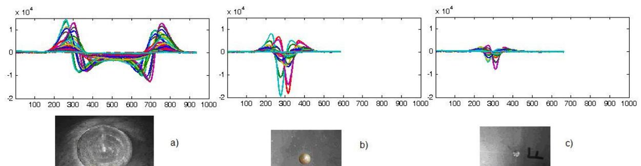
**Figure 1. Signals obtained while scanning over different emulated defects also shown: a) Lake defects of diameter 100mm and depth 2.0mm, b) Conical defect of 16.3mm and depth 3.6mm, c) Pipe defect of 6.0mm of diameter and depth 4.0mm.**
