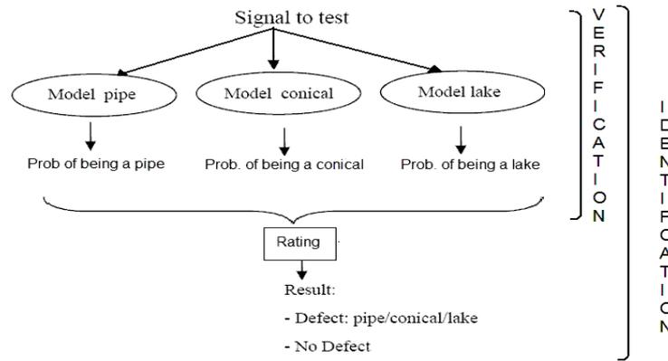
**Figure 5. Scheme showing the experimental procedure**
