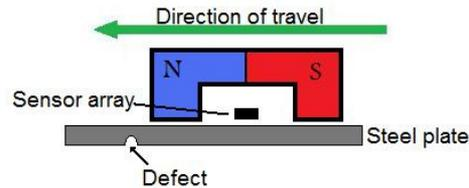
**Figure 1. MFL-based scanning system with permanent magnet moved across a steel plate**
