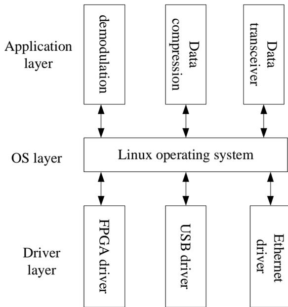
Fig.4 Software frame on ARM9
