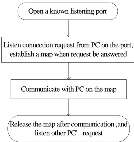
Fig.5 The flow chart of Ethernet on testing box
