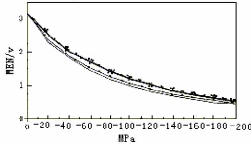
Figure 4 Calibration curve for the relationship between MBN voltage and the stress
