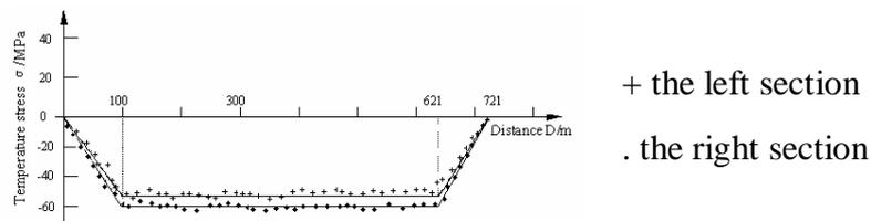
Figure 8. Result 2 of the rail stress testing in the field
