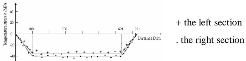
Figure 7. Result 1 of the rail stress testing in the field
