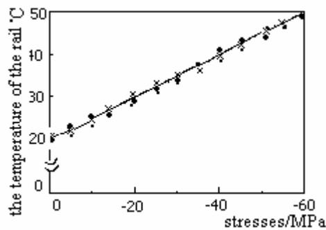
Figure 6. Dependence of temperature against stresses in the sample
