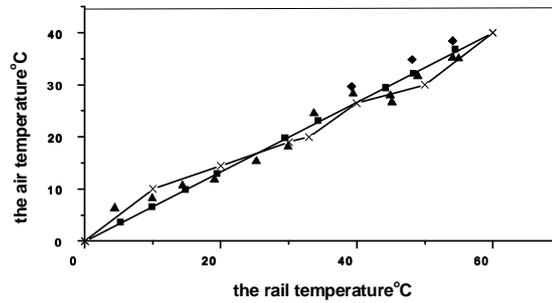
Figure 5. Variation of the rail temperature with the air Temperature
