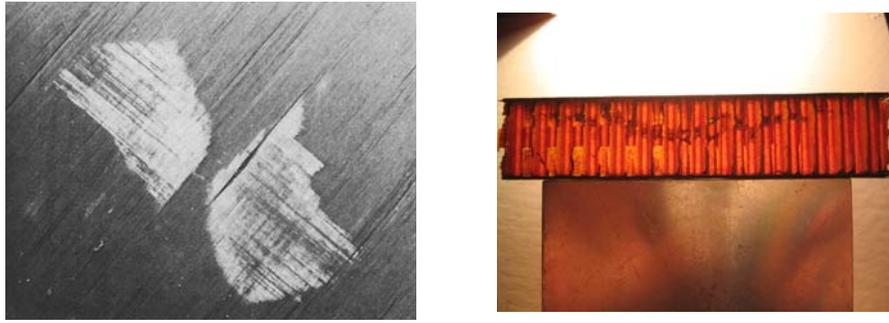
Fig. 2 Two examples of composite damage: delamination caused by impact on solid laminates and core fracture in honeycomb sandwich.
