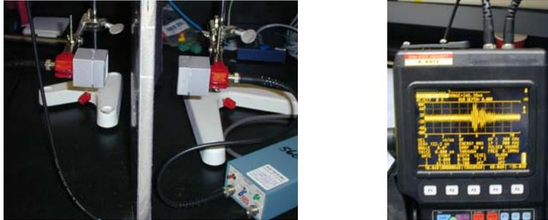
Fig. 8. Detection of disbond in honeycomb sandwich panel with simple air-coupled ultrasonic setup.
