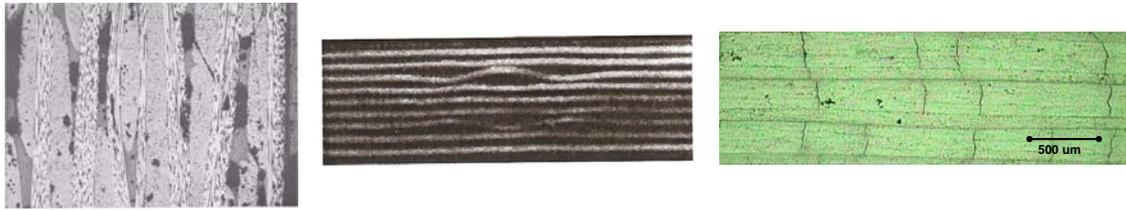
Fig. 1. Examples of defective conditions in composite laminates: porosity, fiber waviness, and microcracking.
