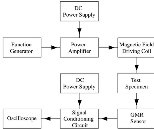
Figure 3. System block diagram of the GMR sensor based eddy current test setup.
