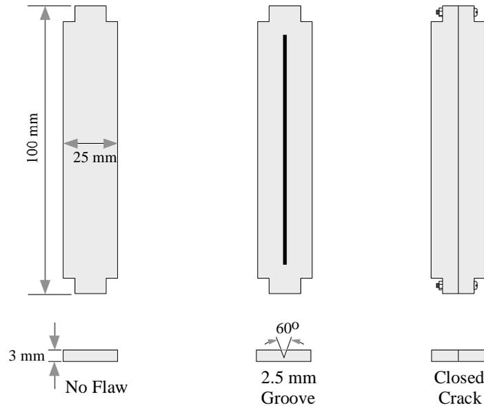
Figure 4. Aluminum 6061 alloy specimens used for Eddy current tests with GMR sensors.
