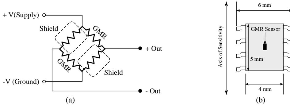
Figure 1. Functional (a) block diagram of GMR Magnetometer sensor, and (b) the integrated package that contains the sensor element.
