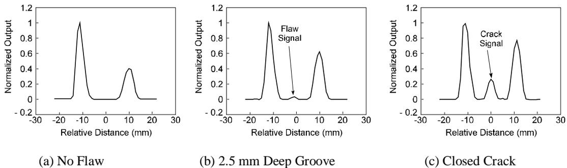
Figure 6. Test results for the stacked aluminum specimens ( $f = 1$  kHz).
