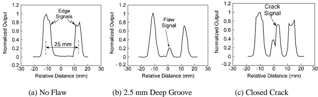
Figure 5. Test results for the single plate aluminum specimens ( $f = 5$  kHz).
