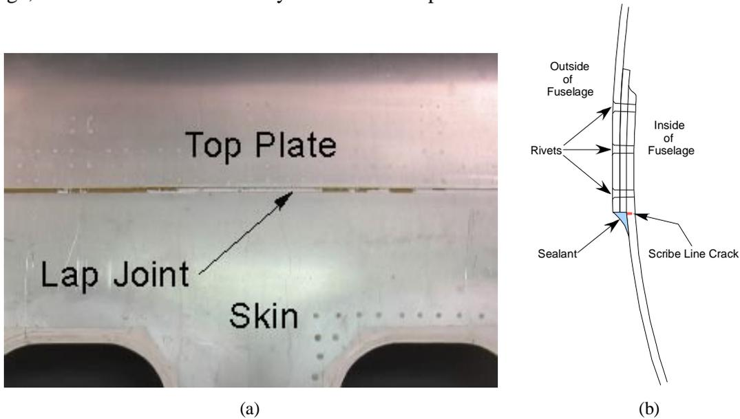
Figure 7. A digital photo of (a) a painted aircraft lap joint and an illustration for (b) its cross-sectional view.
