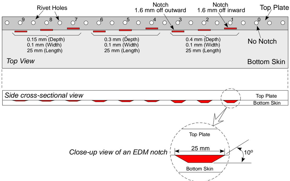
Figure 8. Detailed schematic drawing for the EDM notched test specimens.
