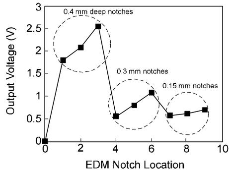
Figure 9. Test result for a typical Boeing 737 aircraft fuselage lap joint combination, 1.8 mm top plate and 0.9 mm skin, with multiple EDM notches ( $f=8$  kHz).
