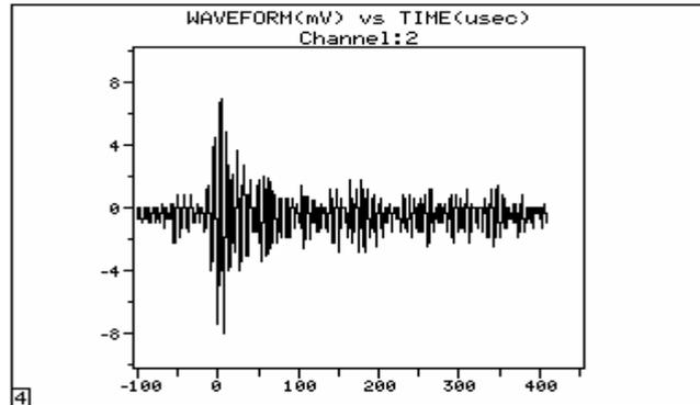
AE source grade is classified on the basis of its strength and activity. Activity is classified as strong activity, activity and weak activity according to the event count in the testing scope during applying and maintaining pressure. Strength is classified as high strength, middle strength and low strength according to the average elastic energy released by the AE event (Table 2 and Table 3).
