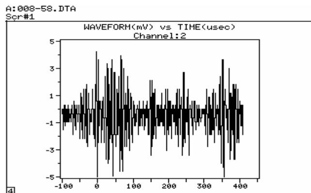
Fig6:Typical continuous signal wave of friction and leak
