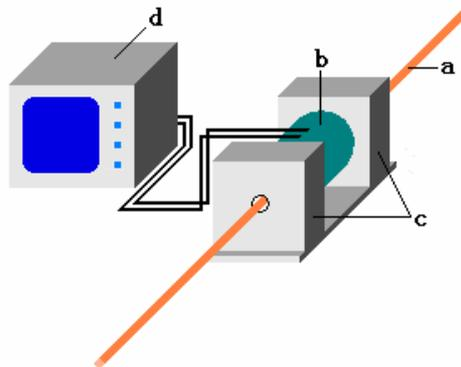
**Fig. 2 EMA guided wave defect testing system for wires**
