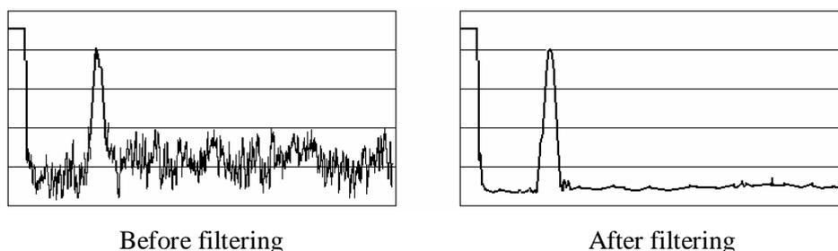
**Fig. 5 Digital treatment of wire testing signal**
