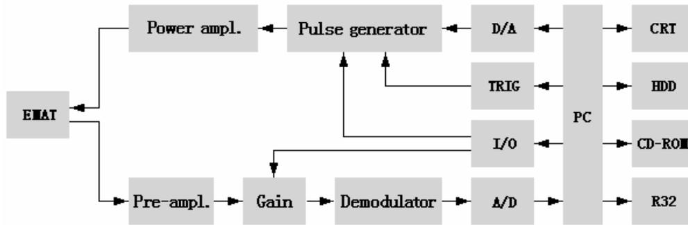
**Fig. 4 Principle block diagram of EMA defect detector**
