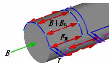
**Fig. 1 Principle of exciting EMA guided wave**
