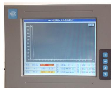
**Fig. 3 EMA defect detector**
