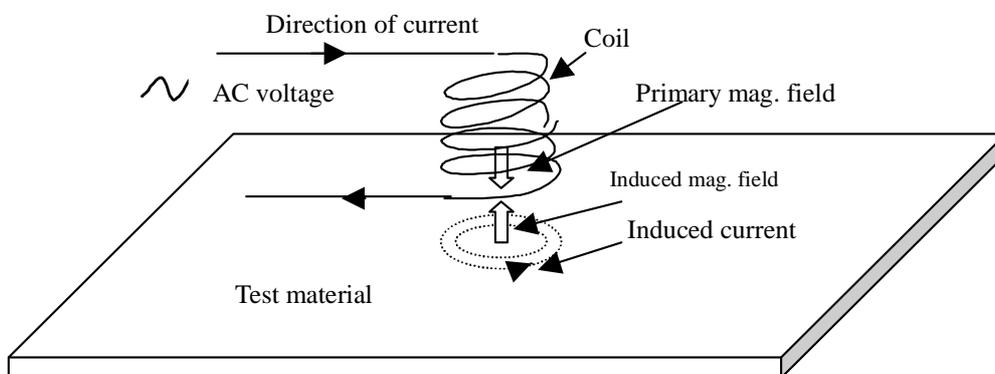
**Fig. 2 Principle of EC testing**
