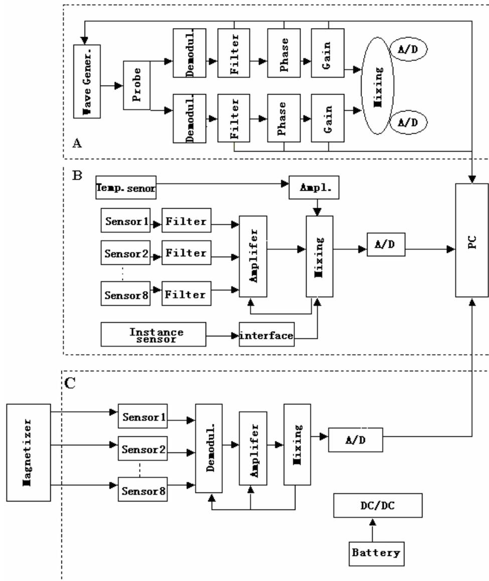
**Fig. 3 Principle block diagram of MMM, EC, MFL Integrated Testing**
