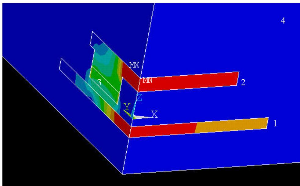
1-plate detected 2- steel bracket 3- Permanent magnet 4-the air layer
