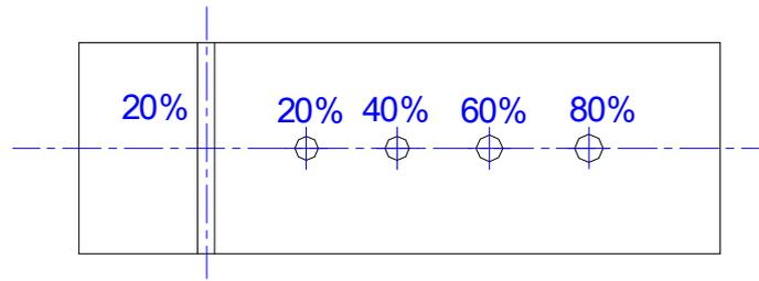
Figure 1 plate magnetic flux leakage test specimen
