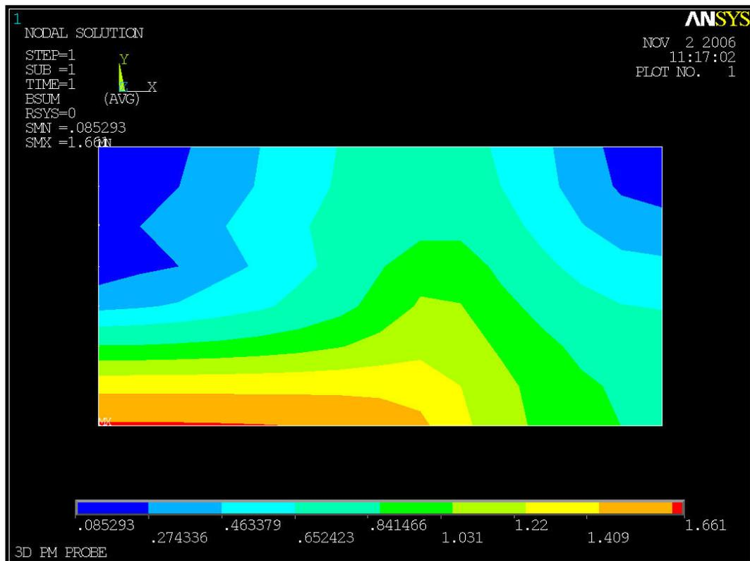
Fig 4 magnetic flux density distribution in plate
