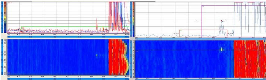
**Figure 8: 2mm FBH 10mm from the bottom (left), 2mm FBH 3mm from the bottom (right),.**
