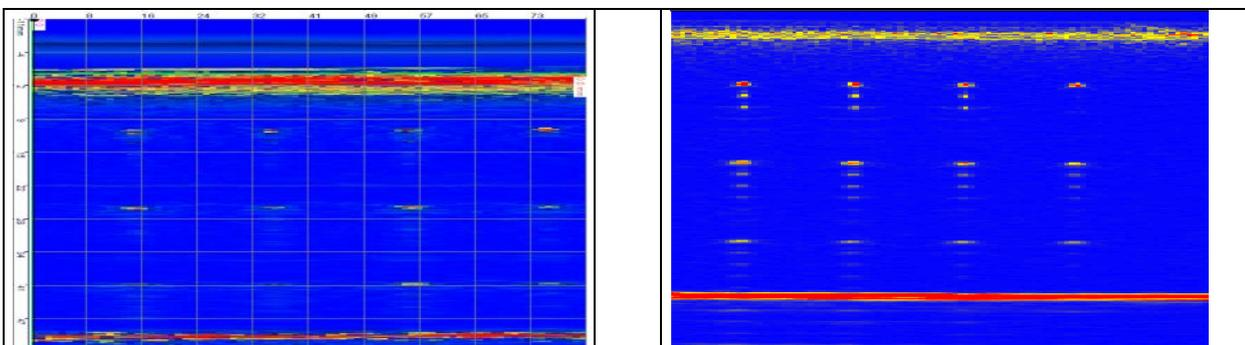
Figure 3. Flaws on the same axis 1. Volume Focusing (Left), Zone Focusing (Right).
