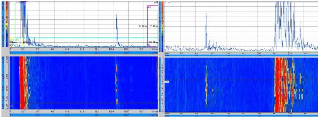
**Figure 10: 4 SDH (2 of 2mm and 2 of 3mm) at 2/3<sup>rd</sup> of the depth of the part (left), 2mm SDH parallel to the section of the part (right).**
