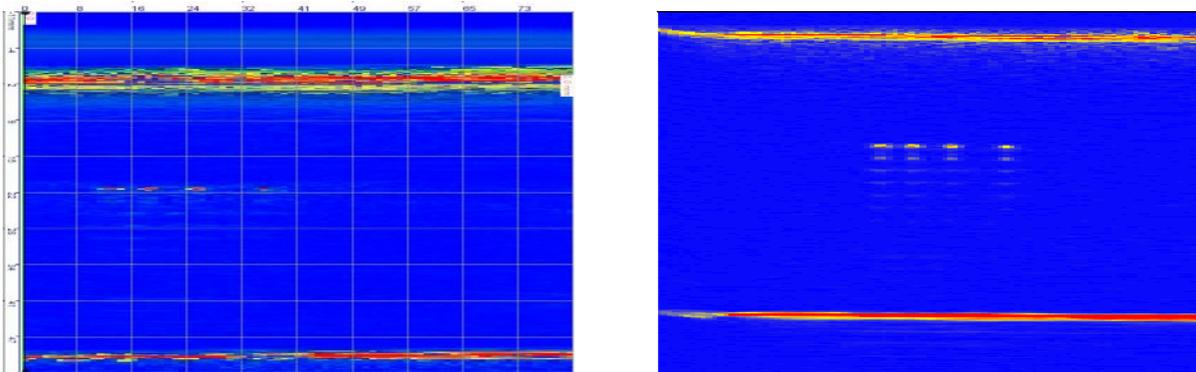
Figure 2. Lateral resolution 1. Volume Focusing (Left), Zone Focusing (Right).
