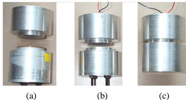
Figure 2. Experiment specimens: (a) Kissing bonds (KB) specimen. (b) Two aluminium-cylinder (Al-Al) specimen. (c) Aluminium (Al) specimen
