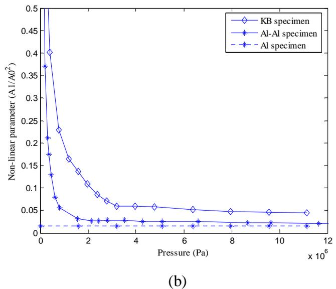
Figure 4. High power ultrasonic response: (a) Non-linear parameter of  $A_1/ A_0^2$  as a function of loading. (b) Zoom in graph of figure 4(a).
