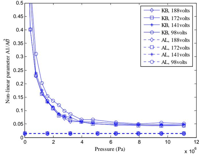
Figure 5. Non-linear parameter  $A_1/A_0^2$  as a function of loading with input voltages from 98 volts to 188 volts.
