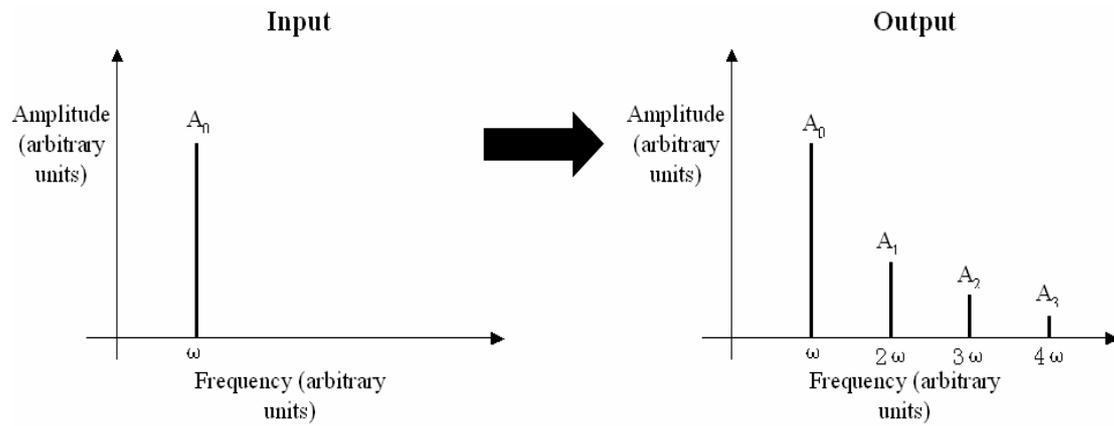
Figure 1. The non-linear behaviour of kissing bonds at the frequency spectrum.
