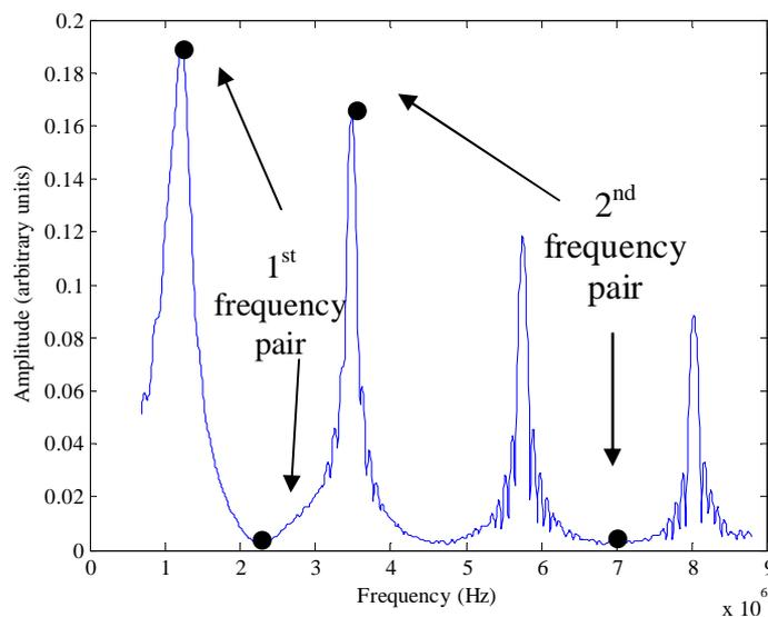
Figure 3. The transfer function of undamped piezoelectric disc
