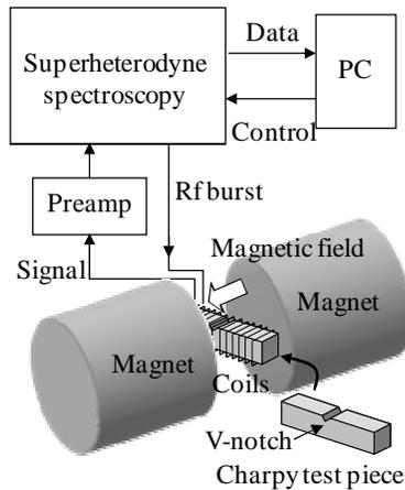
Fig. 5 Schematic representation of the setup for the EMAR measurement.
