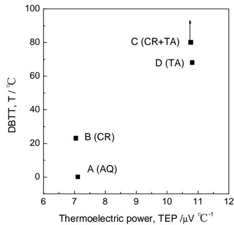
Fig. 4 Relation between TEP and DBTT.
