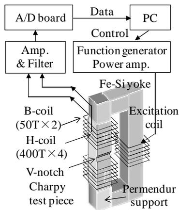
Fig. 1 Schematic representation of the setup for the magnetic measurement.
