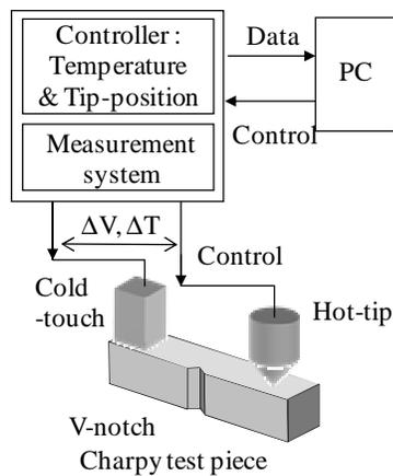
Fig. 3 Schematic representation of the setup for the TEP measurement.
