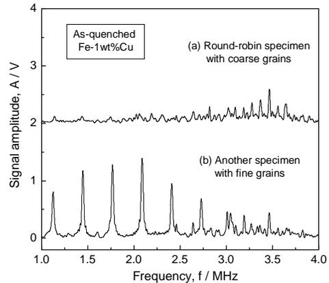
Fig. 6 EMAR spectra of as-quenched specimens.
