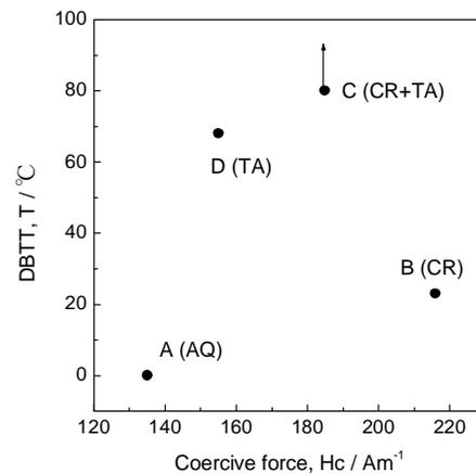
Fig. 2 Relation between coercive force and DBTT.
