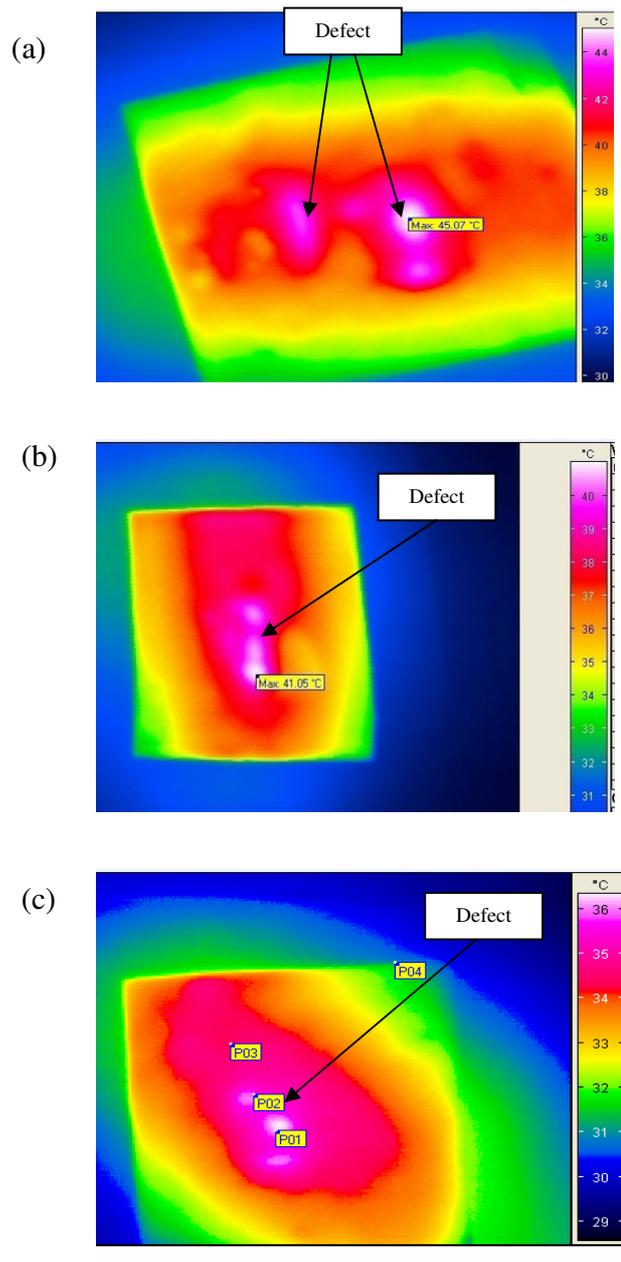
Figure 3: Results of IR thermography for specimens of (a) E-glass/epoxy, (b) carbon/polyester and (c) Kevlar/E-glass/epoxy
