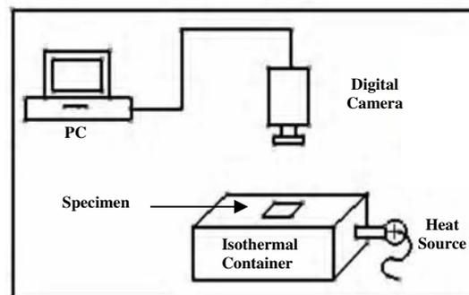
Figure 1: Schematic arrangement for LC thermography
