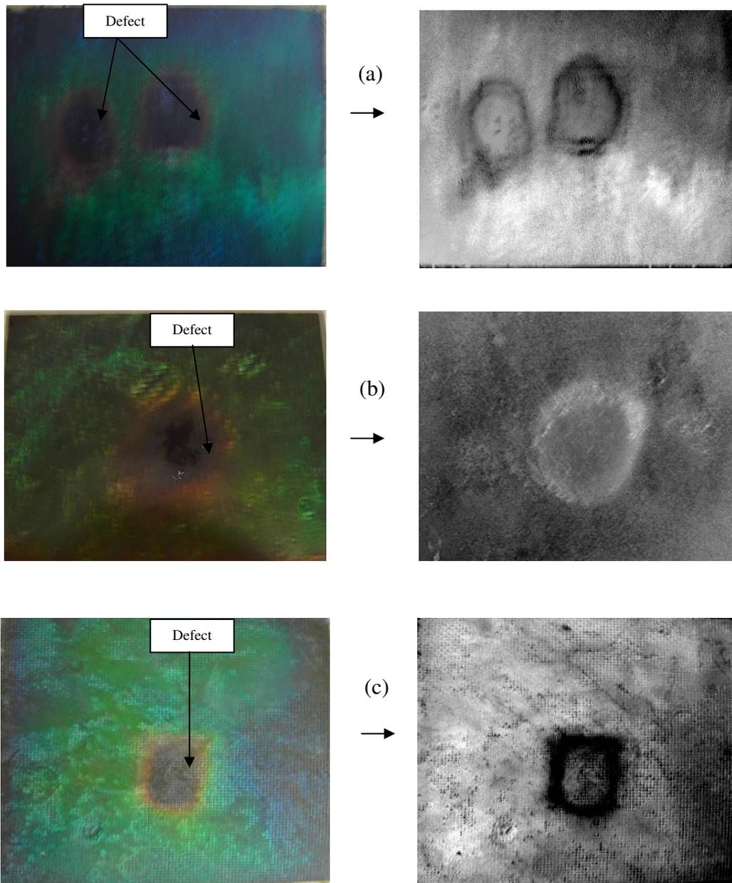
Figure 2: Results from LC thermography for specimens of (a) E-glass/epoxy, (b) carbon/polyester and (c) Kevlar/E-glass/epoxy
