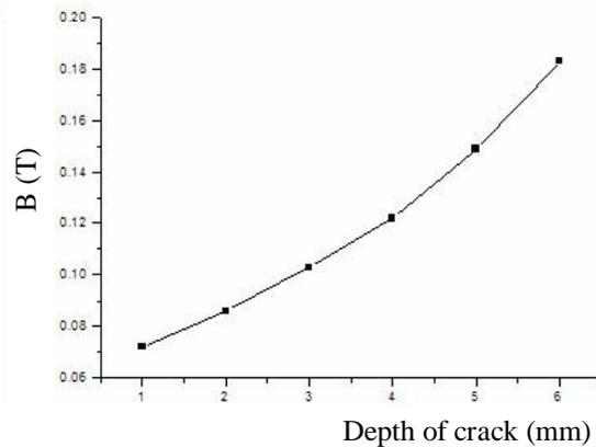
Figure 2. Density of MFL in the cases of different crack depths
