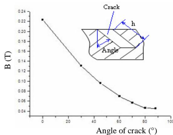
Figure 4. Density of MFL in the cases of different angles of cracks
