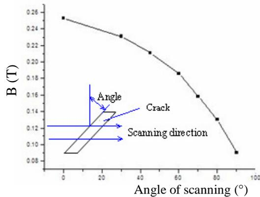
Figure 5. Density of the MFL in the cases of different scanning angles
