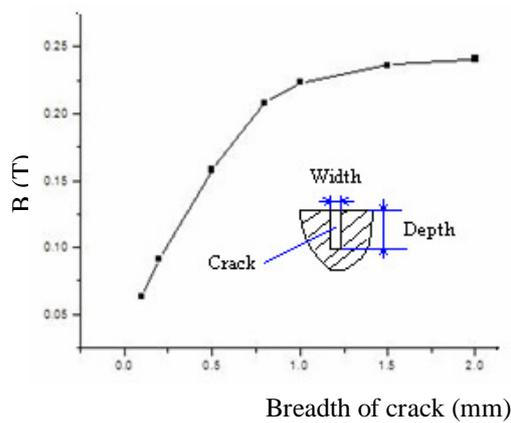
Figure 3. Density of MFL in the cases of different crack widths
