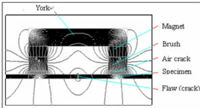
Figure 1. Magnetic flux distribution by 2-D simulation
