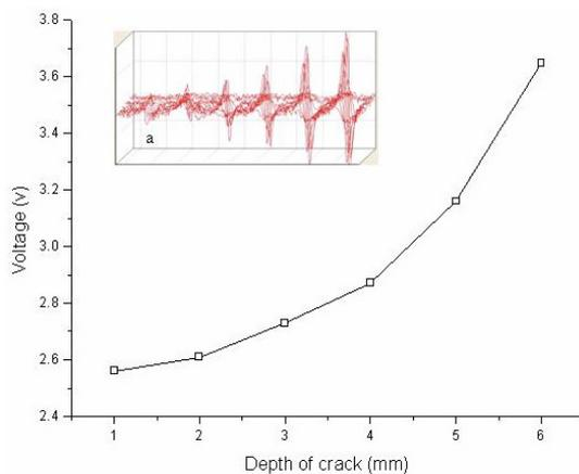
Figure 7. Experiment on crack depth influence a: experimental signals
