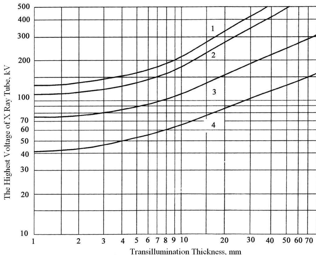
Figure2 The Highest Voltage of X Ray Tube
