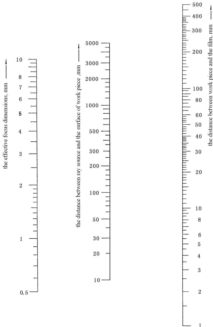
Figure 3 Nomograph for determining distance between focus and work piece at AB level
