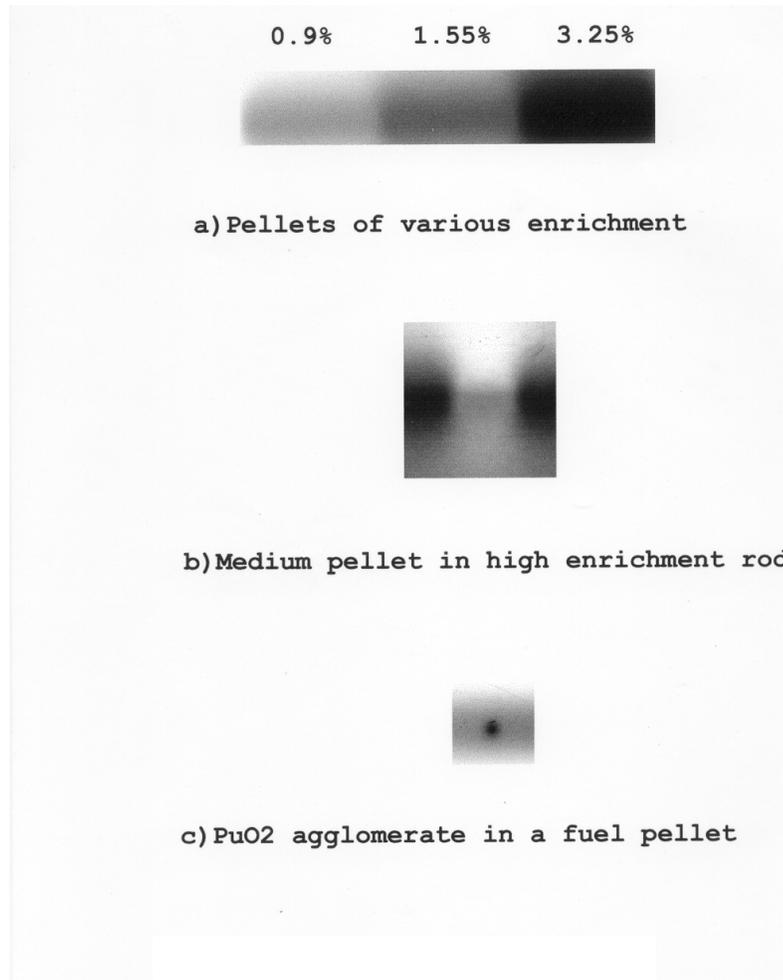
Fig 2. Gamma Autoradiograph of BWR MOX pellets
