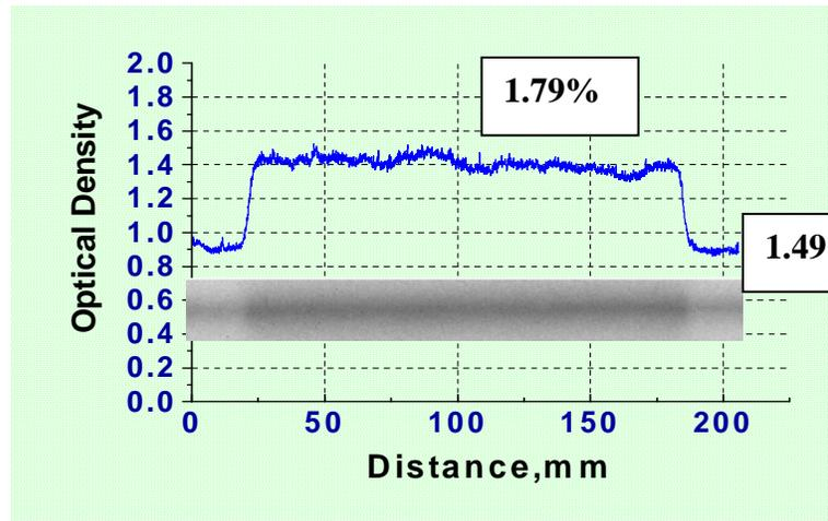
Fig 4 Density scan of GAR showing compositional variation
