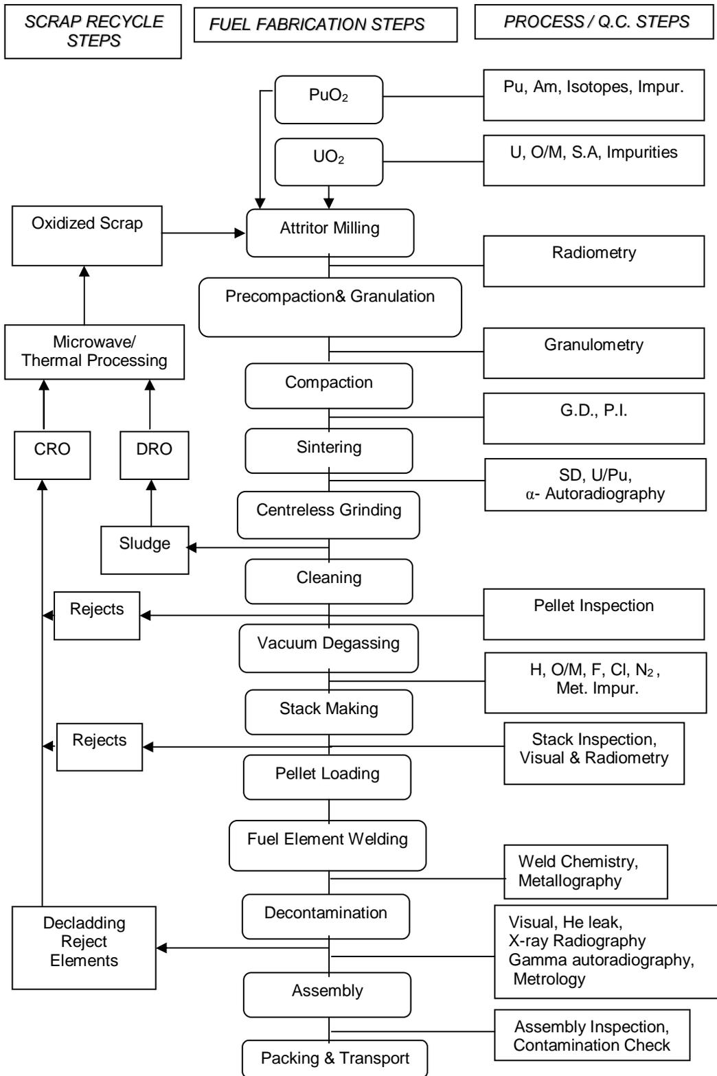
Fig.1 Flowsheet for fabrication of MOX fuel
